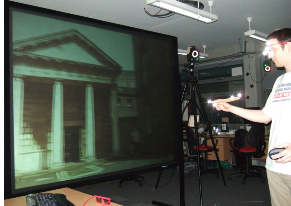
Figure 1: System setup. Two of the Vicon cameras can be seen in the background. The bright glares are the reflective markers.
