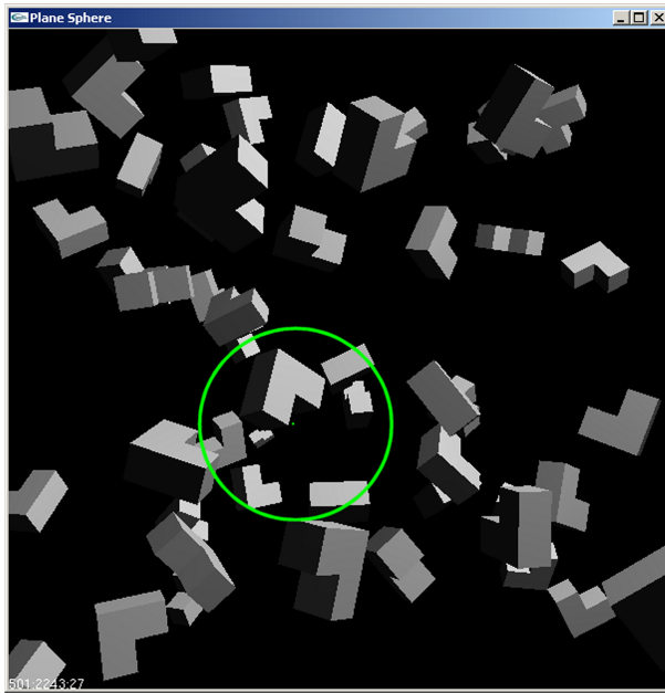
Fig. 15. Collisions inside the region of interest receive more processing time.
