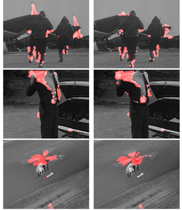
Fig. 2. Each row show consecutive frames from the sequences discussed in Section 3. The detected PM regions are highlighted. In the top sequence the intermittent PM of the propellers and the self-occluding motion of the airmen are detected. The self-occluding motion of the jacket in the 2 nd sequence and the blurred motion of the rotors in the 3 rd are detected.
