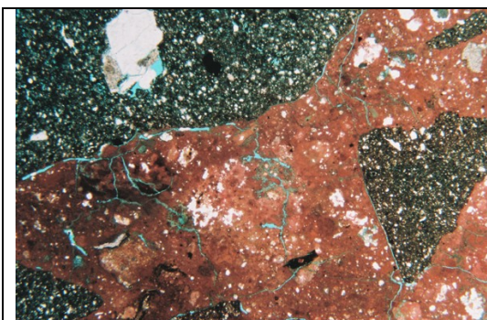
Fig. 11. Brick fragments showing no reaction. Abundant hydrate phases in the lime binder. Celtic mortar, I c. B.C., Inestrillas, La Rioja, Spain. 2X (field of view 4.2mm), natural light.
