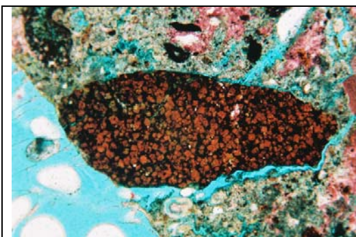
Fig. 5. Coarse remnant of unhydrated ferrite, 19 th century mortars, Dun Laoghaire Harbour, Co. Dublin. Field of view 1.2 mm. natural light.
