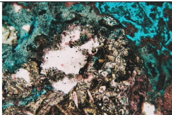
Fig. 8. Amorphous and crystalline hydrates formed in fragment of crystalline rock (probably dolerite), consisting of skeletal olivine and branching plagioclase crystals in a groundmass of plagioclase needles (pozzolanic reaction). Late Medieval lime mortar, St John's Bridge Kilkenny. Field of view 1.2mm, natural light.
