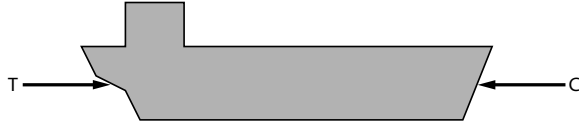
Figure 1: Forces acting on a ship. T is the propeller thrust [N] and C is the drag coefficient.
