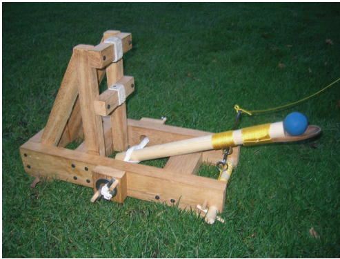
Figure 2. (a) Fully assembled Mangonel complete with “missile” - a squash ball.
