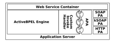
Figure 4. Modified ActiveBPEL Engine
