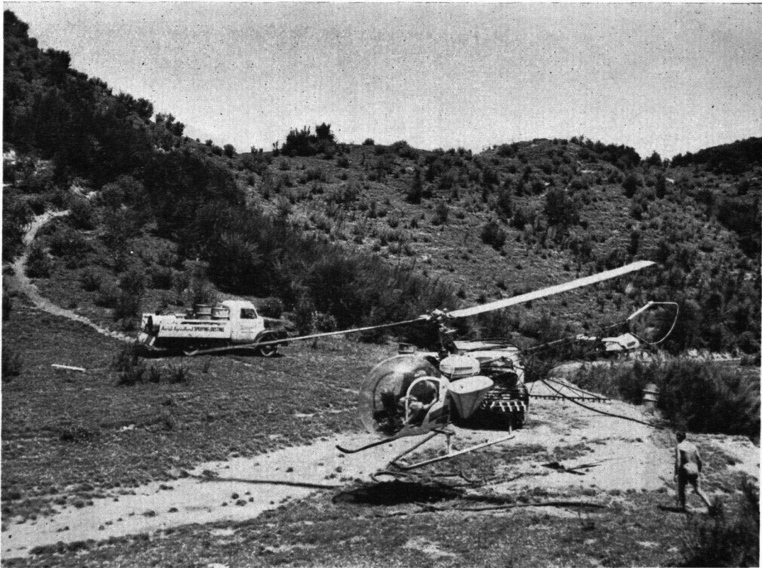
PLATE 5.—Aircraft are also widely used for spraying crops and pests. This helicopter is being employed to spray broom and gorse, which, having been introduced into New Zealand, have become serious pests like other introductions such as the rabbit and deer. The helicopter sprays a 60-foot swathe and the ground is covered four times to give the required saturation for effective killing. The photograph shows the complete service unit filling the tank of the helicopter with the hormone weed killer.
