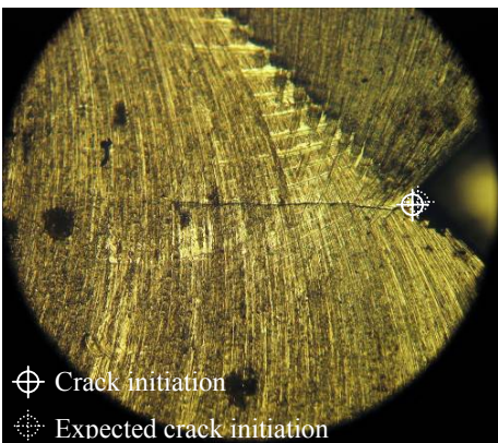
c) Multiaxial test – \delta=1 , \varphi=0^\circ
