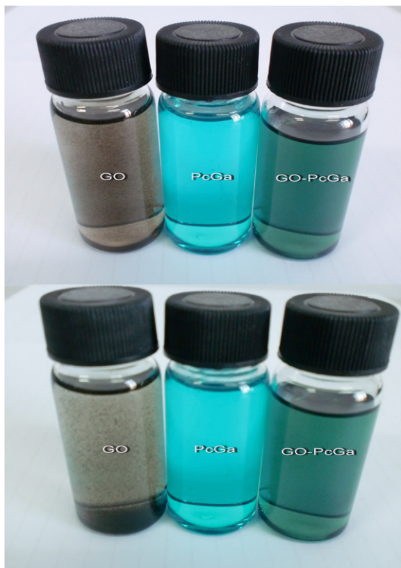
Figure 1. Digital pictures of the samples dispersed in chloroform: (above) dispersions immediately after sonication; and (bottom) dispersions 1 h after sonication. The concentration for each sample: 1 \text{ mg ml}^{-1} .
