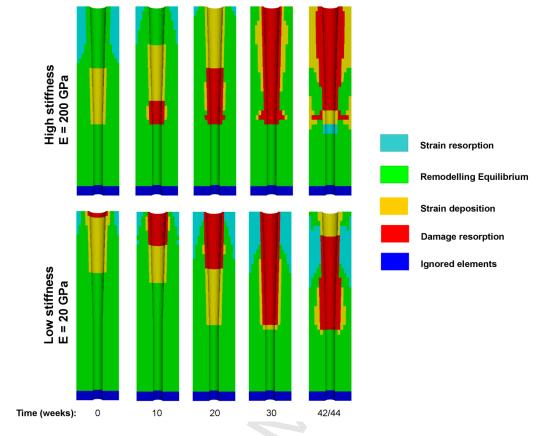
Figure 3: Contour plots of strain and damage activity at different time points during the simulation for the reference ideal 'average' cases for each stem. Note that the reference case is with a bone external diameter of 22.5 mm,  $\varepsilon_{min}$  = 1000  $\mu$ ε and  $\varepsilon_{max}$  = 2000  $\mu$ ε.
