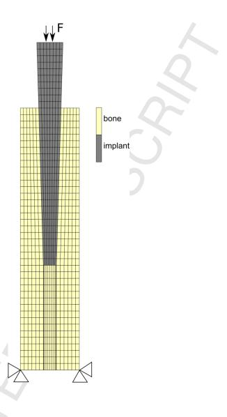
**Figure 1:** A 3D finite element mesh of an intramedullary implant of the reference
