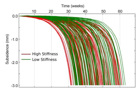
**Figure 6:** When all analyses are run (100 per implant, therefore 200 in total) very significant variation is in subsidence is predicted. Statistical analysis shows that there is no statistical difference between the performance of the implants (refer to Table 1).
