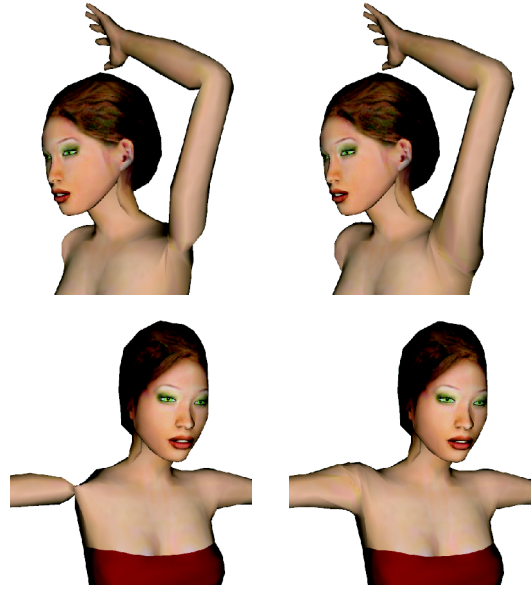
Figure 7: Comparison of linear (left) and dual quaternion blending (right). Dual quaternions preserve rigidity of input transformations and therefore avoid skin collapsing artifacts.
