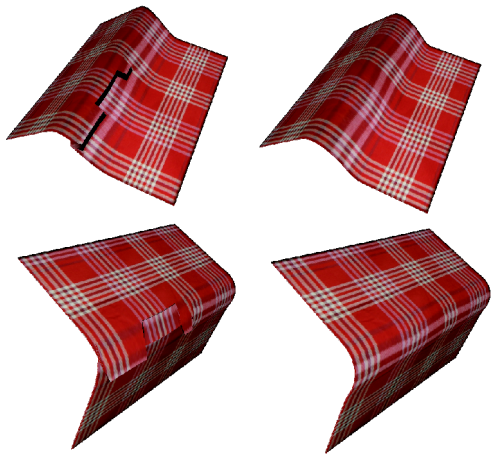
Figure 8: Comparison of direct quaternion blending (left) and dual quaternion blending (right). Only the latter delivers smooth deformation.
