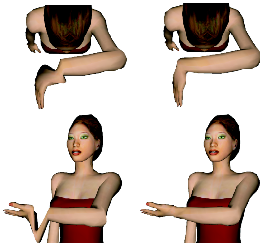
Figure 9: Comparison of log-matrix (left) and dual quaternion blending (right). The shortest-path property of dual quaternion blending guarantees natural skin deformations.
