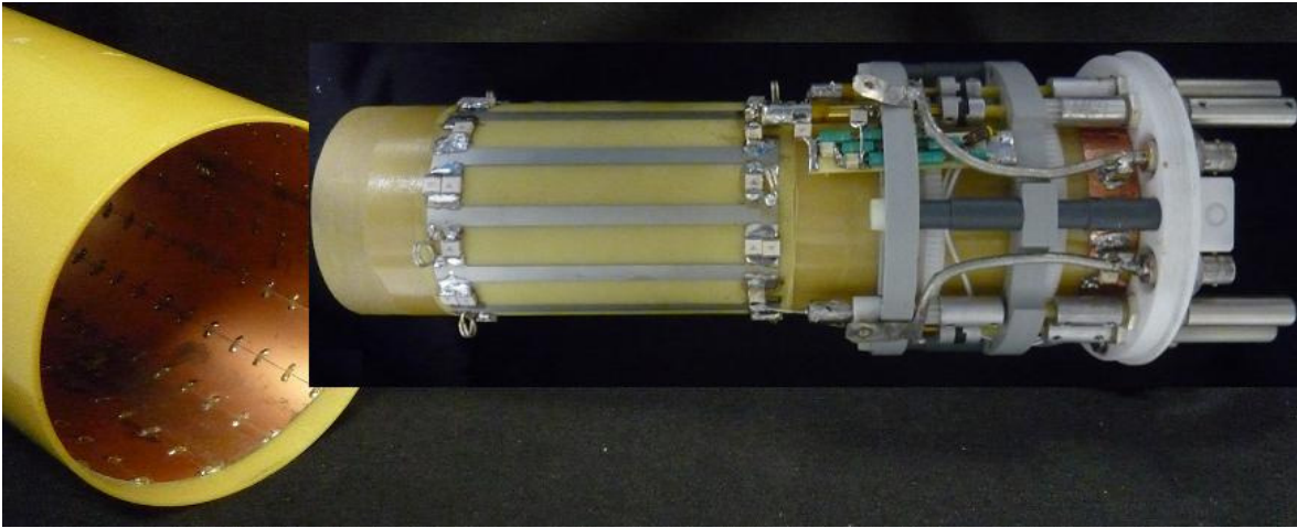
Figure 5.8: The newly-developed resonator system composed of the RF-shield and the ^1\text{H}/^{23}\text{Na} birdcage coil (inset).
