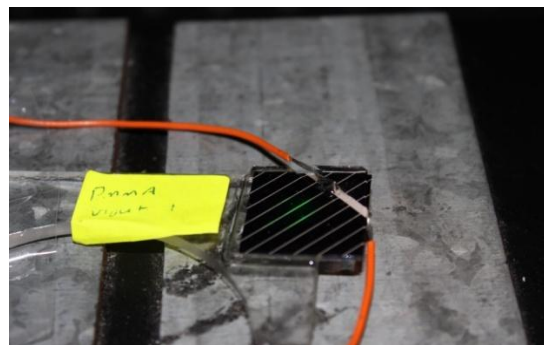
Figure 2: Si cell encapsulated with an LDS layer of Lumogen Violet/PMMA.
