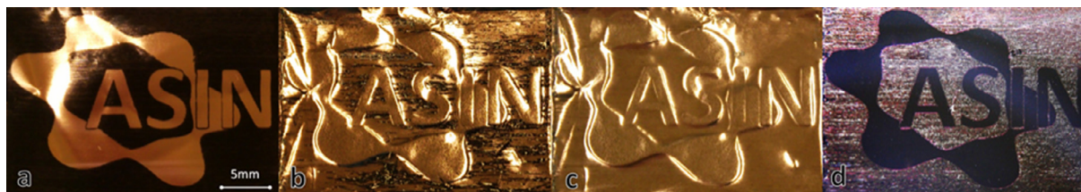
Fig. 2 – (a) Cu foil that has been prepatterned with the inverse pattern; dark (inked) areas will not grow graphene, bare copper will; (b) the same foil after CVD growth; (c) after mild sonication and (d) graphene pattern transferred to SiO 2 wafer. (A colour version of this figure can be viewed online.)
