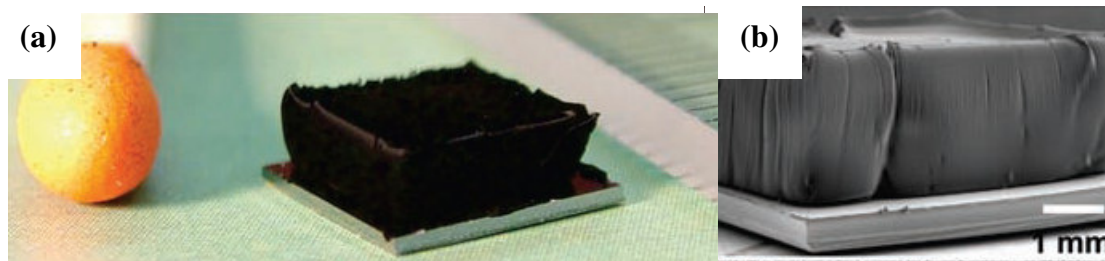
Figure 2.9 (a) Optical and (b) SEM images of SWNT forests produced by supergrowth [47] .
