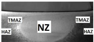
Fig. 2 Zonal microstructure of FSW (Adapted from [1])
