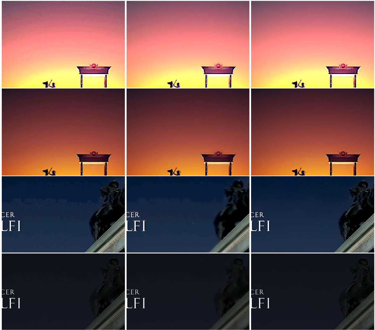
Figure 7: Left column: Frames from the Memphis ( 1280 \times 720 ) and House of Cards ( 1920 \times 1080 ) sequences. Center column: The result of gradfun technique. Right column: The result of our deband technique. Contrast enhanced images are in the odd rows.
