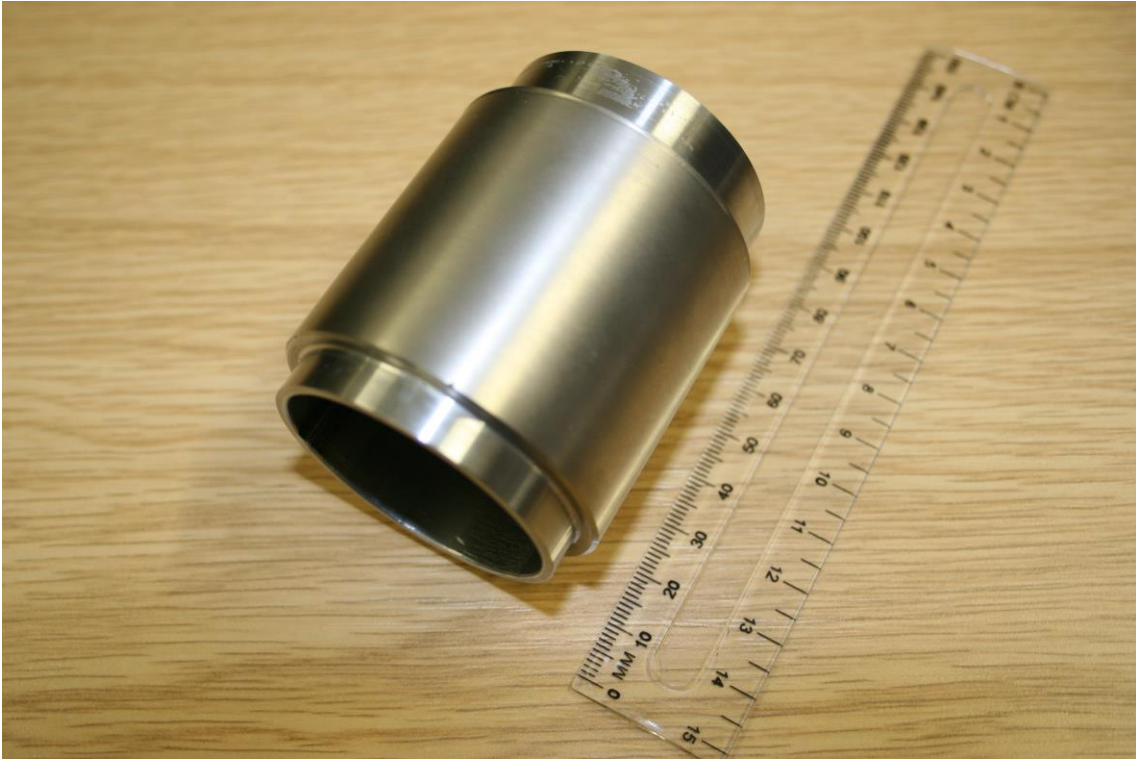
Figure 4: Thick titanium coating (3mm) on a steel tube by SLD.
