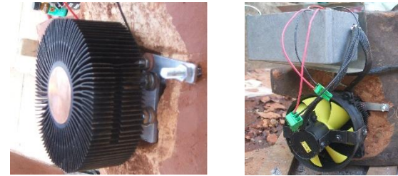
Figure 5: Mounting of the generator's heat sink and circuit box to the stove wall
