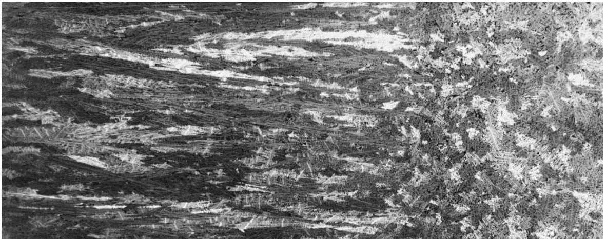
Fig. 2.4 Columnar to equiaxed transition visible in a longitudinal section of a cylindrical sample (70 mm in diameter and 150 mm in length) of Al–7wt.%Si [47].
