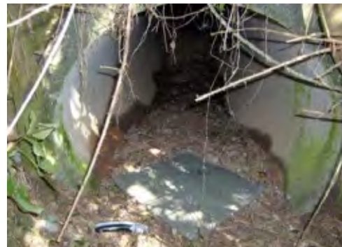
Figure 1. A clay mat installed at the entrance of a badger tunnel to monitor use by mammals.
