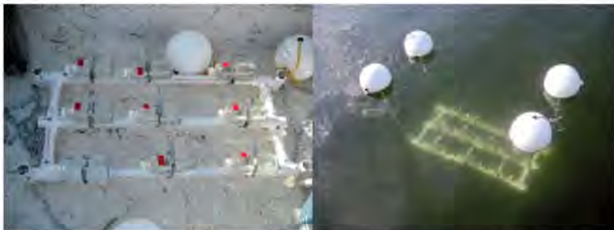
Figure 3. Study Apparatus With Bottles Used to Suspend Stormwater Samples in Water Column (left). Apparatus With Samples Incubating in Hillsborough Bay (right).
