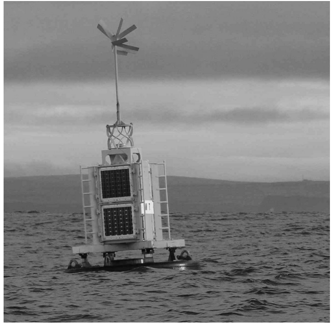
Figure 1. A buoy during calm conditions - note solar panels and communications antennae
