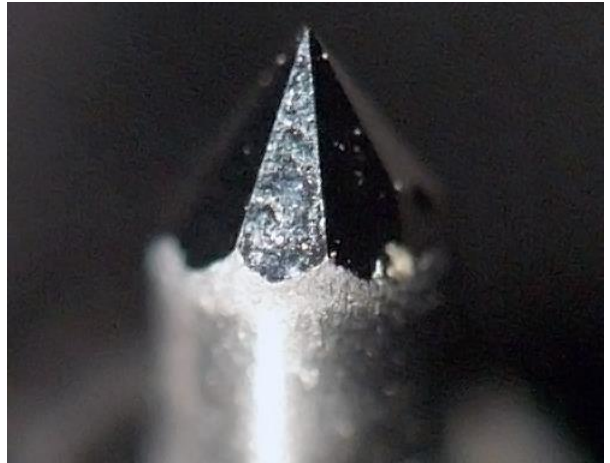
Figure 1. A \langle 111 \rangle -oriented single crystal boron-doped diamond probe with a properly shaped pyramid at the apex. The diameter of the diamond tip is 1 mm.
