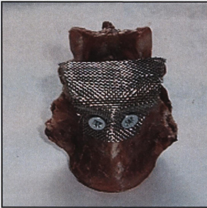
Figure 3.9. Anchored mesh plate with two screws inserted through the plate into the vertebral body 6mm below the endplate.
