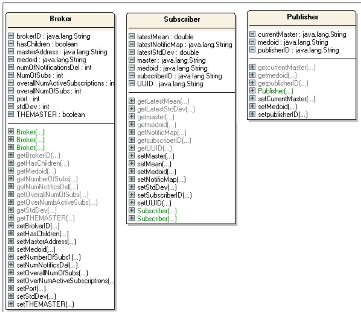
Figure 17: UML Class Diagrams for Broker, Publisher and Subscriber
