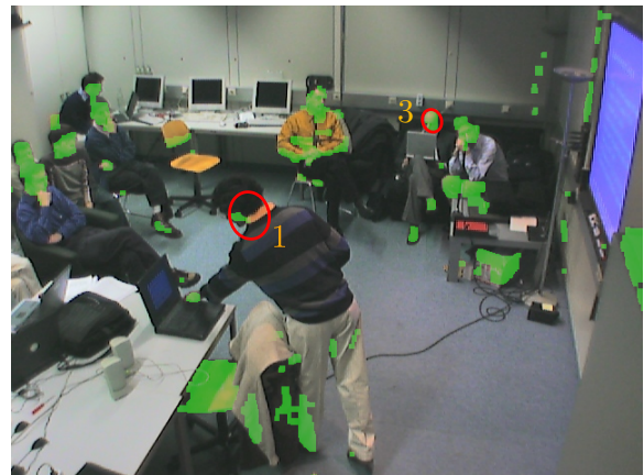
(d) Camera 4: Skin colour mask with example detected heads.
