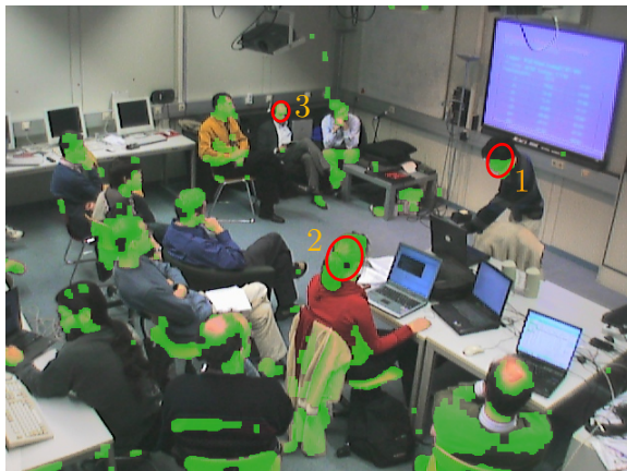
(c) Camera 3: Skin colour mask with example detected heads.
