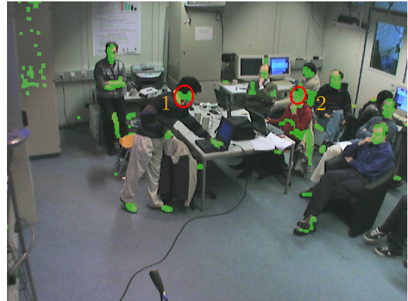
(b) Camera 2: Skin colour mask with example detected heads.
