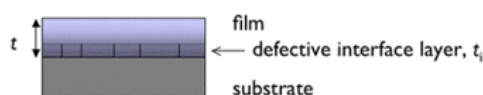
Figure 5.4. Simple schematic depicting a possible origin of RTFM in MB 6 thin film nanostructures due to an interfacial defect-rich layer residing at the thin film-substrate interface.
