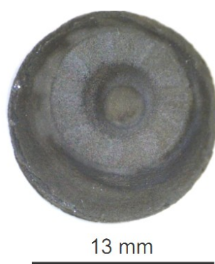
Figure 2.4. High resolution optical image of a BaB 6 target used for PLD; pitting due to the impact of the of the focused laser beam on the surface can be seen.
