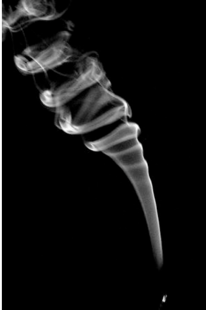
Figure 3.2: Cigarette smoke as it rises develops turbulent characteristics (photo credit: Cigarette smoke, Pal & Basu).
