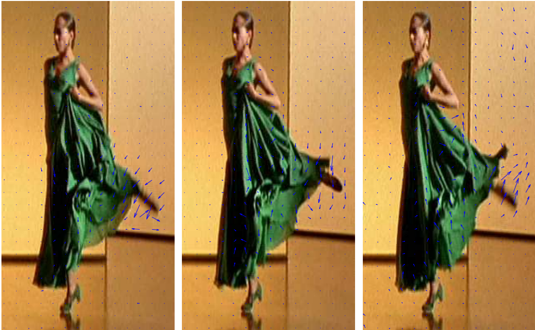
Figure 6.17: An edit point and the local motion vectors pertaining to it. The change of direction in the dancer’s foot is clearly reflected in the vector field in that region. The vectors shown are backward motion, at a blocksize of 17x17.
