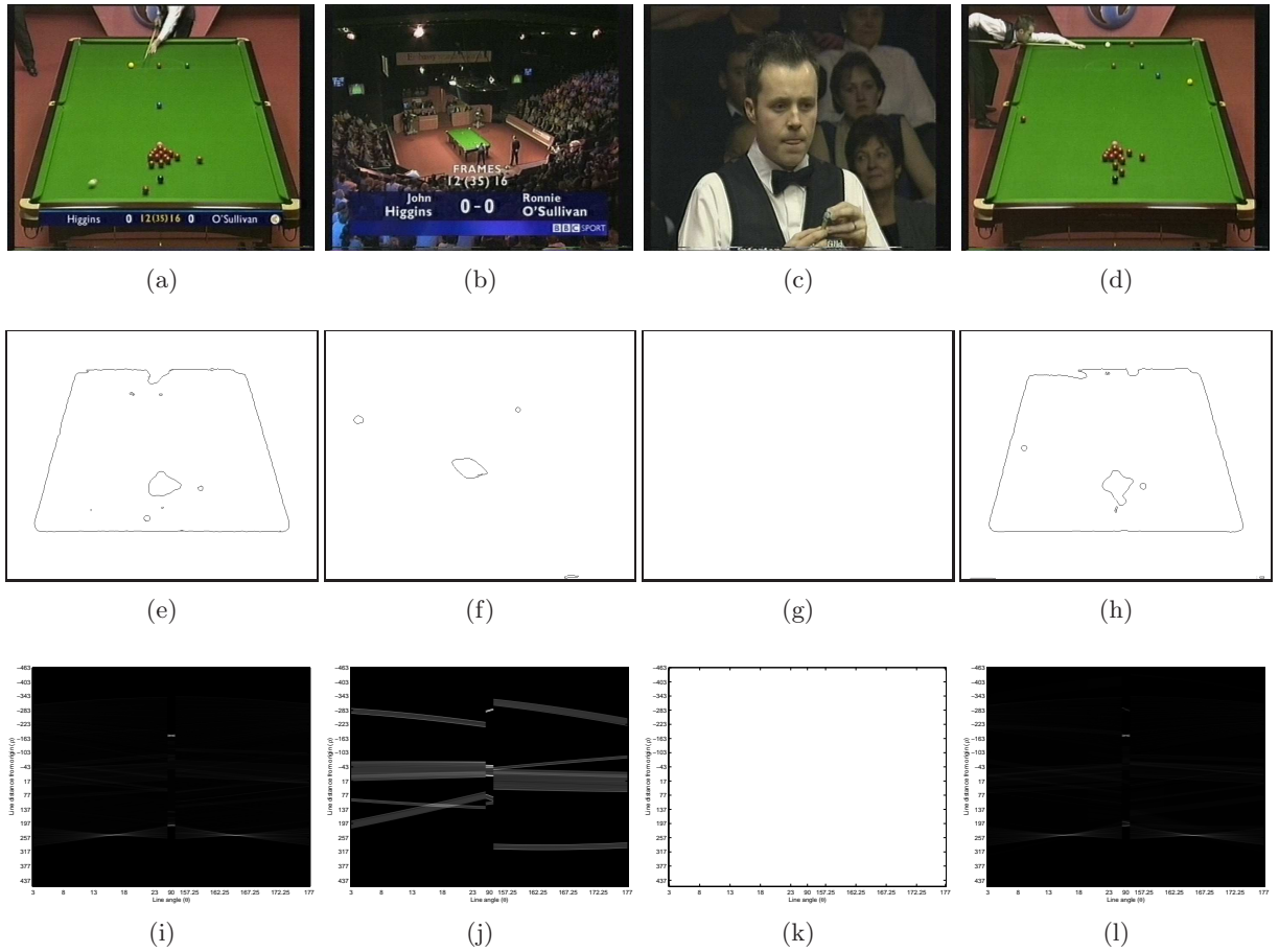
Figure 5.3: Examples of table finding. The top row shows original frames from the snooker footage. The middle row presents the edges found in the green mask. In the bottom row, the Hough transforms of these edge maps are shown. The characteristic four-peak pattern is present only in those frames containing the full-table view.
