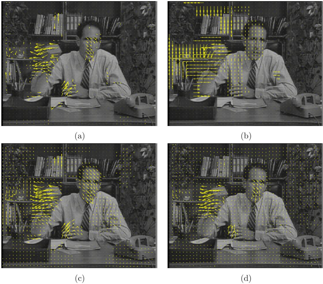
Figure B.9: Salesman sequence (8x8 Blocks). (a) WBME result. (b) 3DRS result. (c) ICM smoothing. (d) BP smoothing.
