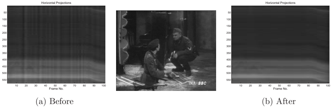
Figure 6.13: Horizontal temporal projections of tunnel sequence (a) before and (b) after flicker stabilisation.
