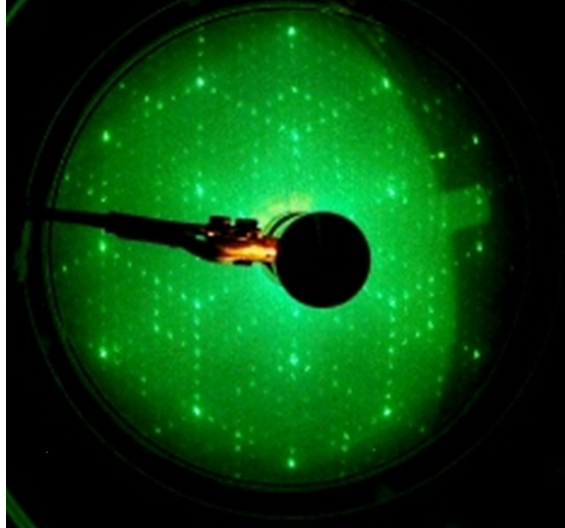
Figure 3.6: LEED image, viewed from the rear, taken from the clean Si(111)-7×7 surface.
