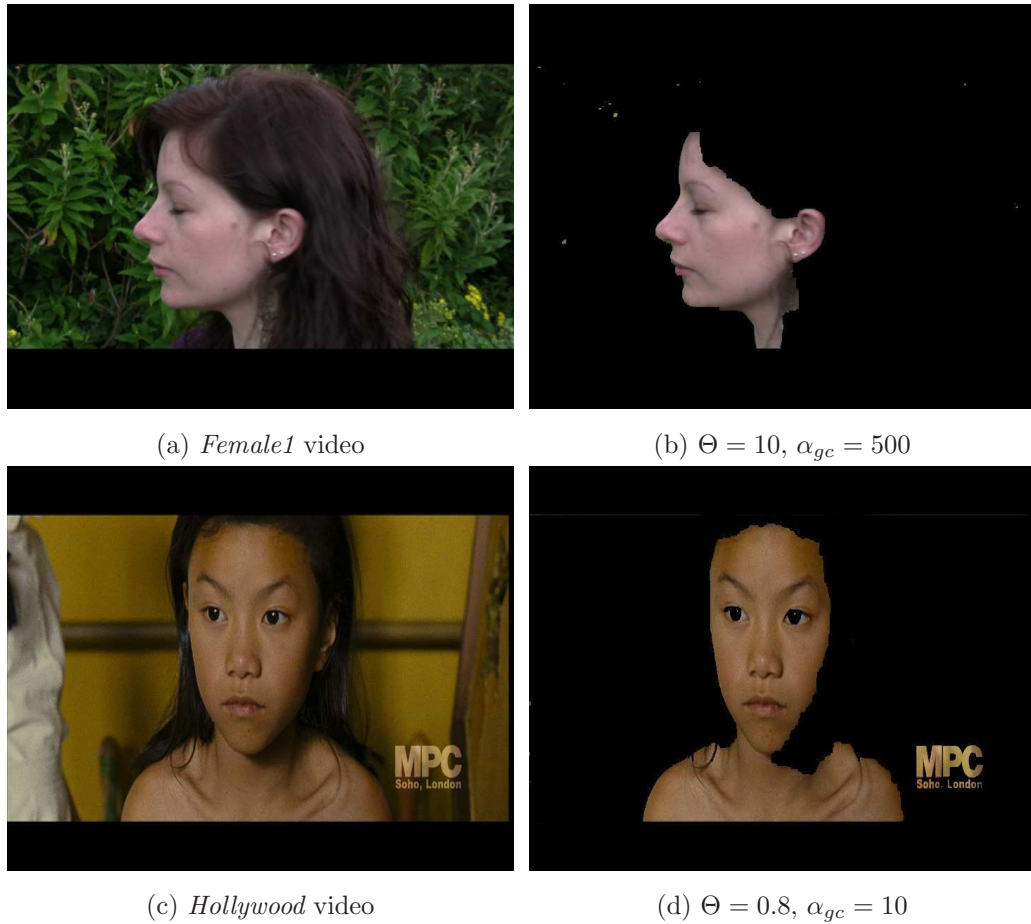
Figure 5.3: Graph Cut-based skin segmentation; (a) a single frame of source video Female1 , (b) binary skin segmentation with \Theta = 10 and \alpha_{gc} = 500 , (c) single frame of source video Hollywood , and (d) binary skin segmentation with \Theta = 0.8 and \alpha_{gc} = 10 .
