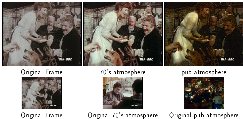
Figure 3.7: Example of Colour Grading for Image and Video Restoration. It is possible to recreate different atmospheres. Here an old faded film is transformed to match the colour scheme of a movie from the 70’s and a pub ambiance.
