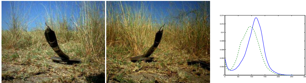
Figure 4.3: Example of Radiometric Calibration issue on a outdoor multi-camera footage. The image on the right is darker which results in a shift to the left in the intensity histogram (dashed green plot).
