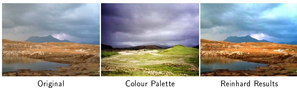
Figure 3.2: Example of Colour transfer using Reinhard [Rei01] Colour Transfer. The transfer fails to re-synthesise the colour scheme of the target image. To be successful the method would require human interaction.
