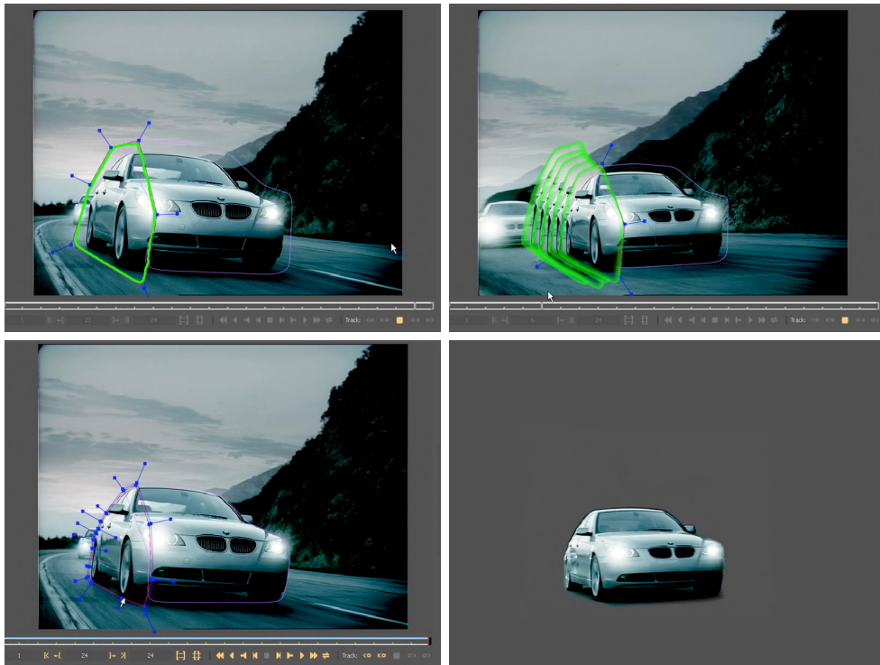
Figure 5.11: Example of planar tracking in Imagineer Systems’ “Motor”. In the first image, a coarse region (corresponding to the side of the car) in frame 23 is selected to be tracked (green). Second image, the user assumes a perspective motion model, and allows the system to track the region backwards through the sequence (to frame 6), warped in-between regions are shown in green. Third image, a more accurate set of roto curves are placed in the same region at frame 23. The motion parameters from the region track are applied to the accurate curve set. A separate track is calculated (and used to drive another refined curve set) for the front of the car (as it is assumed the side and front of the car are allowed to deform separately). Last image, the accurate matte in frame 6 is created entirely using the backwards propagated roto information. (Images courtesy of Imagineer Systems.)
