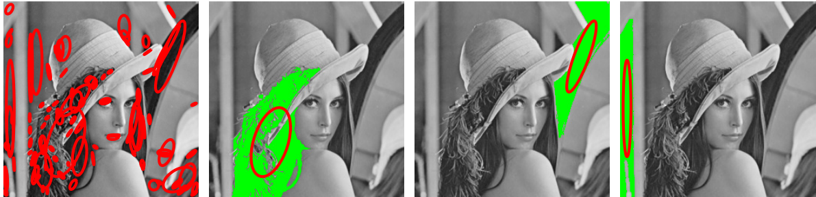
Figure 2.7: Left, example of all ellipses detected on the image, using a connectivity tolerance of \delta = 2 . Images two to four show the three largest detected connected components in the image and their associated ellipses (the MSER implementation demonstrated here is that of Vedaldi [175]).
