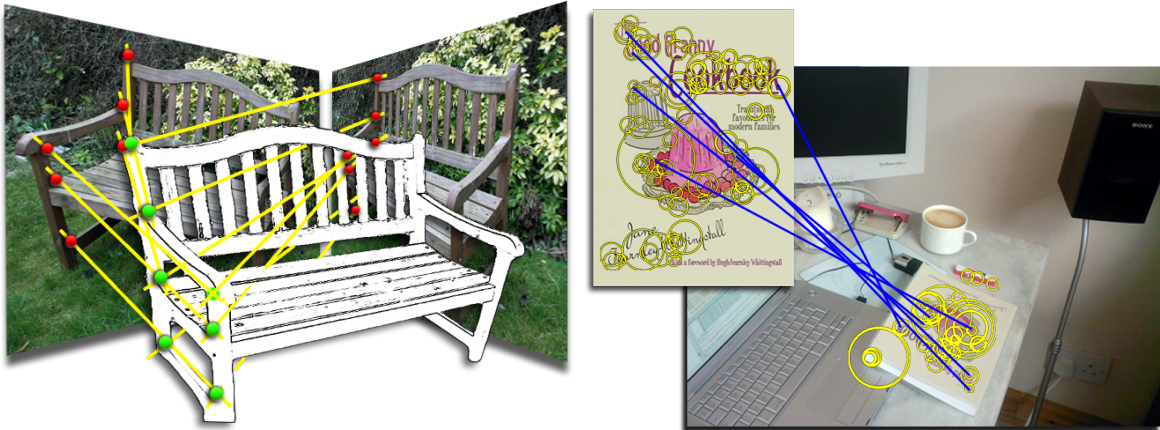
Figure 2.1: Examples of correspondence matching. Left, correspondences between features in a pair of images (red) are used to estimate depth, allowing the shape of the object to be recovered in 3D. Right, features calculated between a query image and desktop scene (yellow circles) are matched (blue) to allow detection and localisation of the book cover despite changes in object scale, rotation and scene illumination.
