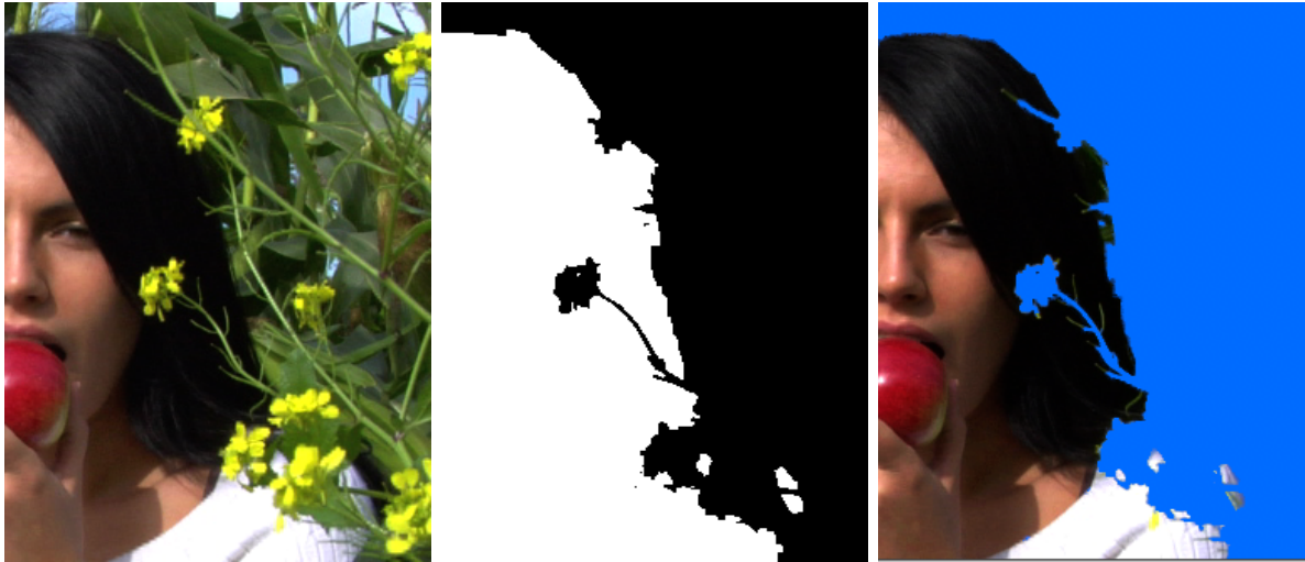
Figure 6.16: Close-Up of results from the “Lady Eating Apple” sequence. From left to right; original, matte from algorithm, non-binary matte composite onto blue background. Despite the intricate shapes of the plant’s branches, an accurate matte can be found. Notice however, that some finer plant branches were not segmented. During the manual segmentation of the object in other frames, the same fine structures were not selected by the user, and so have not been segmented by the algorithm. Whether strong fidelity to the user mattes is good or not is a matter of taste.
