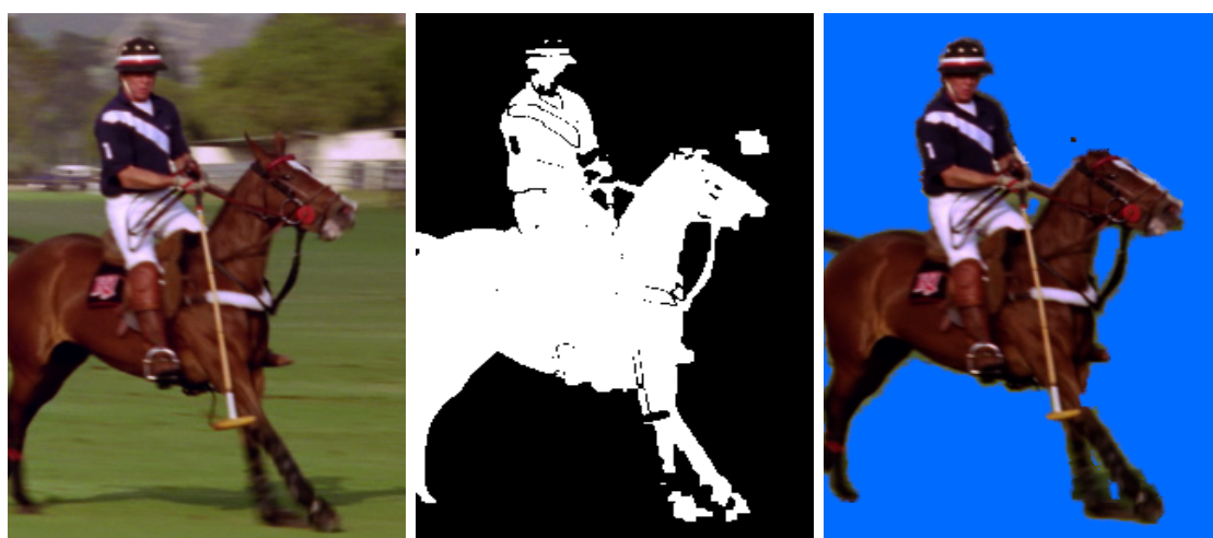
Figure 6.21: Example of the algorithm failing on the “Polo” sequence. The low number of feature correspondences between this frame and those with user-supplied mattes (mostly due to motion blur) has caused a number of missing regions on the horses legs, ears. Visible in the centre image, a number of incorrect feature matches have introduced blotches falsely accepted as object, and caused part of the helmet and jersey to be falsely labelled as being background. Notice that the non-binary matte (right) can compensate for a lot of mistakes, but the result is still not perfect. For example, the ears are still missing, due to low colour contrast. Again, in this case the user would need to manually touch-up the matte.
