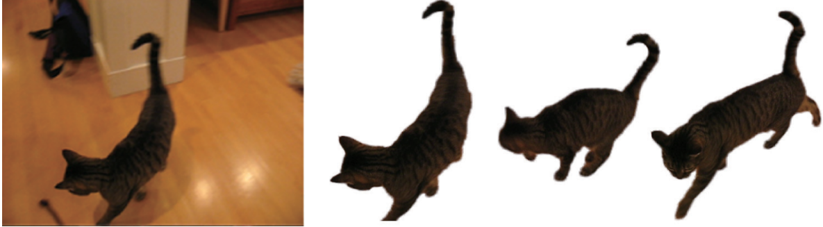
Figure 5.20: Example of results obtained by the LIVEcut system of Price et al. Three segmented example frames are shown from the “Cats Playing” video. This sequence is difficult for many reasons, such as objects in the same scene with similar colour (the rope, the other cat, and the background shadows), multiple complicated motions (from both cats and camera motion), and large changes in object topology (the cat’s legs, tail and ears). These difficulties would usually cause traditional systems to fail or require heavy corrections. However, the high quality segmentation results obtained by the LIVEcut system show the effects of combining many complimentary feature cues effectively. (Images courtesy of Price et al.)
