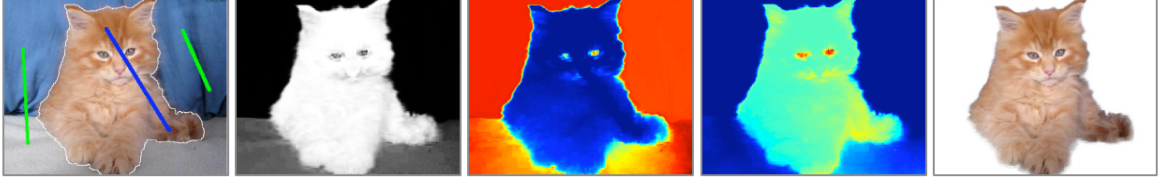
Figure 5.9: Example of using the Distance-Cut system. The user begins by drawing object (blue) and background (green) scribbles (1 st image). The system calculates the label likelihood for each pixel from the object and background colour distributions (object colour likelihood, P_F(\mathbf{x}) , shown in 2 nd image). The likelihoods are then used as weights in the object and background geodesic distances (3 rd and 4 th images, blue is low distance, red is high). The labelling at each site is given by the class with the minimum geodesic distance at that site (last image). Note that the colour likelihood in the second image is probably good enough to allow segmentation without using geodesic distances. (Images reproduced from Bai & Sapiro [10].)
