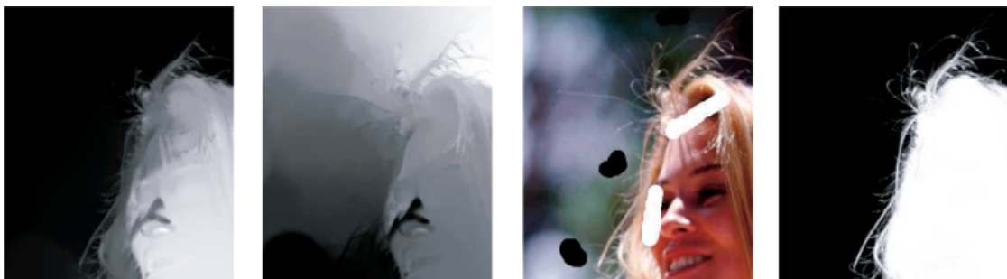
Figure 5.26: Analysis of the first two smallest eigenvectors (first two images) yield the optimal placement for user background and foreground scribbles. Regions with similar grey level values are considered connected. In the third image, scribbles are drawn in the “coherent regions” (of smooth appearance) in the eigenvector images. Last image, the resulting matte of only using eigenvector analysis to decide scribble placement. (Images reproduced from [92])
