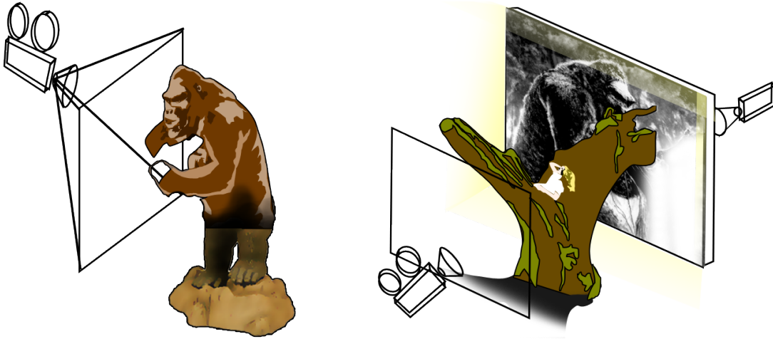
Figure 5.2: Early “in-camera” matting for cinema. To composite “King Kong” into real footage, the stop-motion animations were first filmed (left), then projected onto a large screen behind the real set (right). This is referred to as an “in-camera” process as no additional manipulation of the film is needed for the composition.
