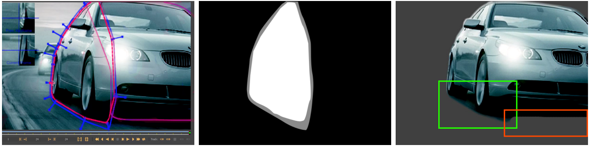
Figure 5.21: Example of matting using roto-scope curves in Imagineer System’s “Motor” BMW sequence, the goal is to create a smooth segmentation around the shadow and the road. Left, an ambiguous area is specified using two curves (inside and outside, red and blue respectively). This is known as “feathering”. Centre, a “tri-map” is calculated as the difference between one of the two roto curve pairs, where definite object is shown in white, definite background in black, and the “unknown” region in which the non-binary labelling is to be calculated, shown in grey. Right, the effect of the non-binary label assignment process is shown in the green square. The red square shows the cut out results in the absence of feathering. Notice how the feathering produces a soft, non-binary edge along the shadow of the car, giving a more realistic look than the binary cut out shown in the red square. (Images courtesy of Imagineer Systems.)
