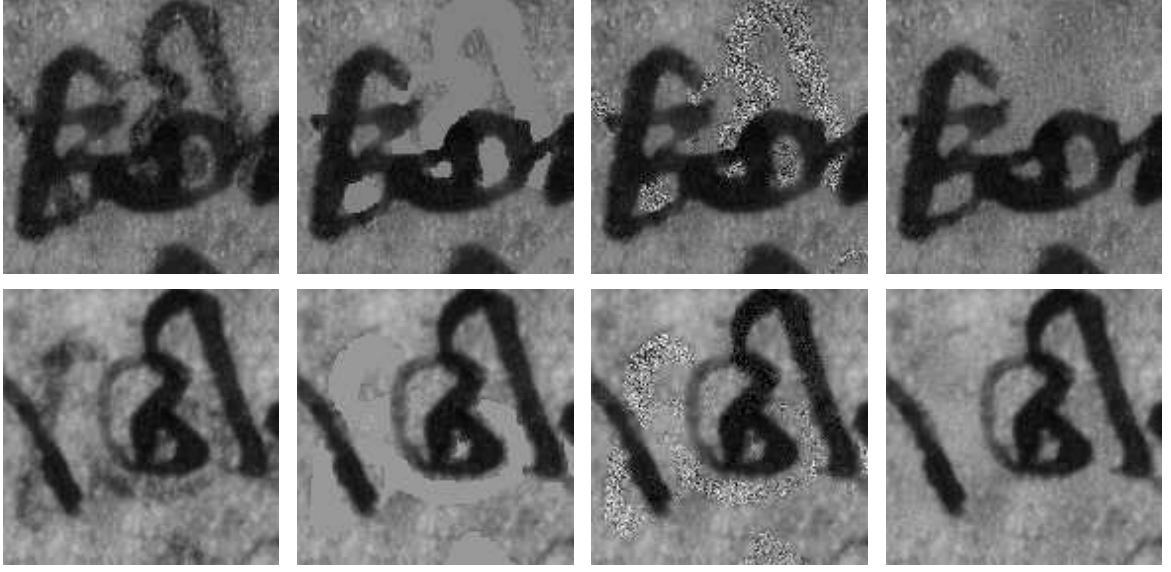
Figure 3.4: Drawing samples to estimate the clean images produces better results visually. Left to right: Original degraded recto (top) and verso sample images, clean image estimates (with known foreground masks) using the mean, unconstrained random samples, and constrained samples of the error distributions. M19 .
