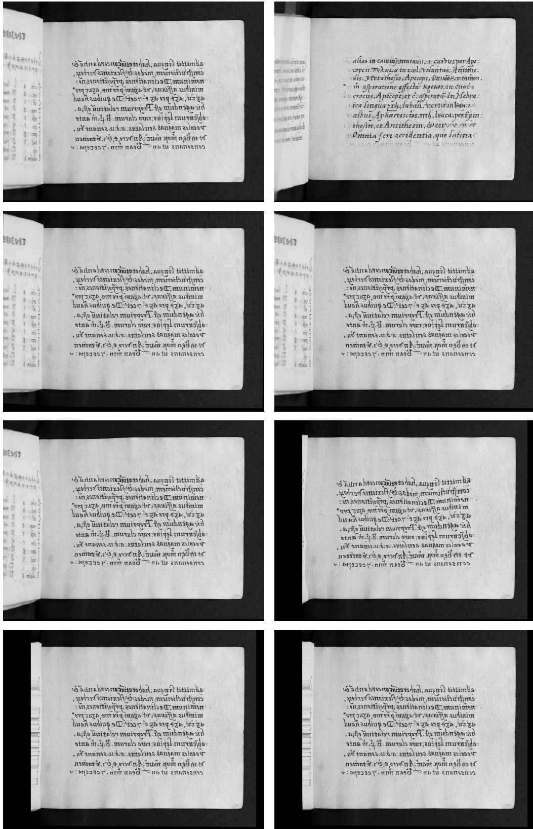
Figure 6.11: Comparison of registered results for image 21, M02, where the visible width of each side of the page is different. Top row: reference image J (left), warped image I . 2nd row: manually registered image (left), result for Method 1. 3rd row: Results for Methods 2 (left) and 3. Bottom row: Results for Methods 4 and 5.
