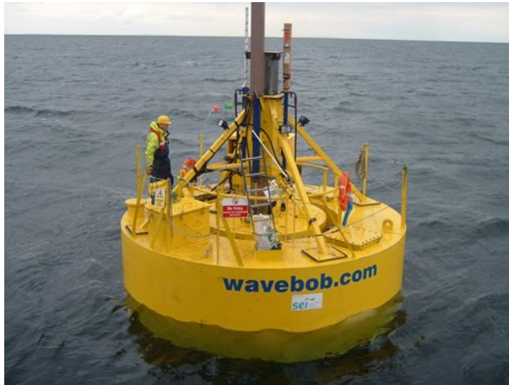
Figure 2.7: 1:4 scale Wavebob model at sea [21]
