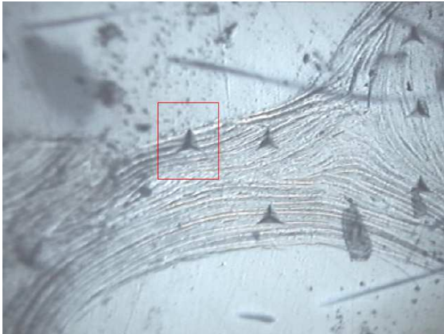
Figure 3.8: Indentation set showing indentations performed close to embedding medium. Left-most indentation deemed too close to sample edge.
