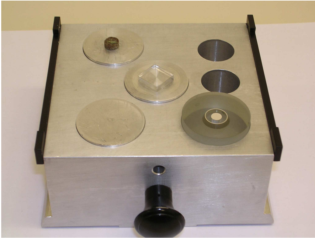
Figure 3.2: Sample stage with bone sample, aluminium standard and fused silica standard inserted.
