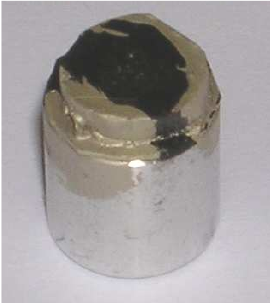
Figure 3.10: Embedded trabecular bone sample mounted on aluminium SEM stub with silver paint placed around the circumference.
