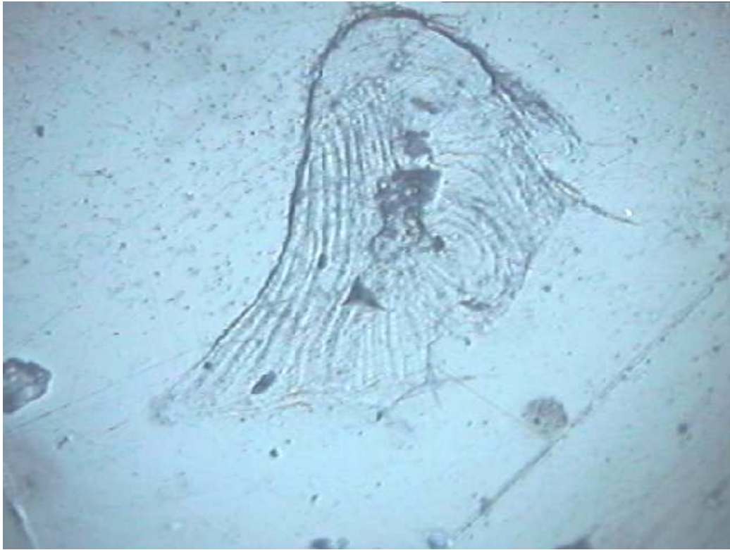
Figure 3.7: Trabecular bone sample showing insufficient depth of material, imaged using light microscopy with specimen embedded in PMMA.
