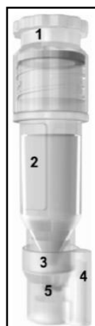
Figure 2-15: Schematic Diagram of Flash-memory Chip Equipped Cryovial (Ihmig et al., 2009).
