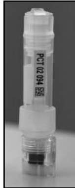
Figure 2-14: 2ml Cryovial Equipped with Barcode, RFID and Flash-memory Chip (Shirley et al., 2009)
