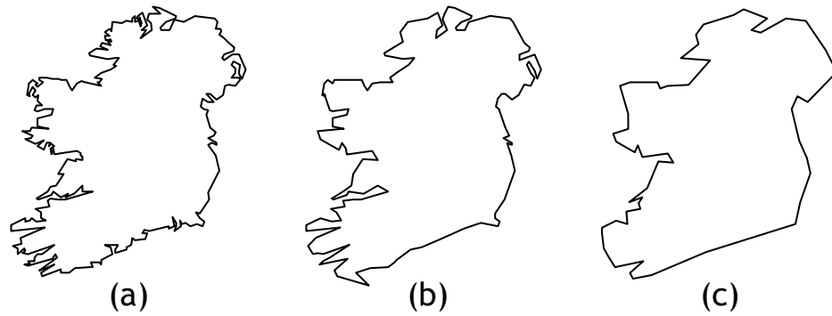
Figure 3.10: Simplification generalisation step
