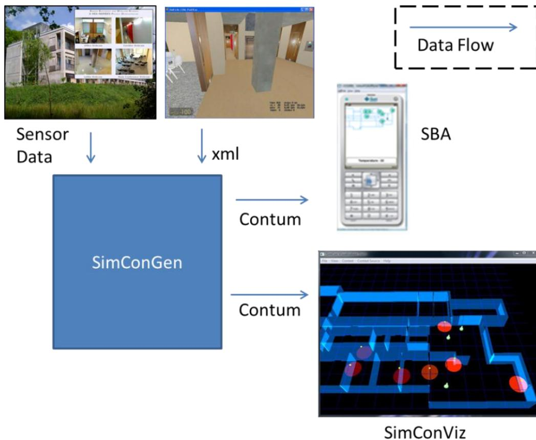
Figure 5-17 Displaying Hybrid simulation, simulated coordinate and real temperature using SimConGen and SimConViz.
