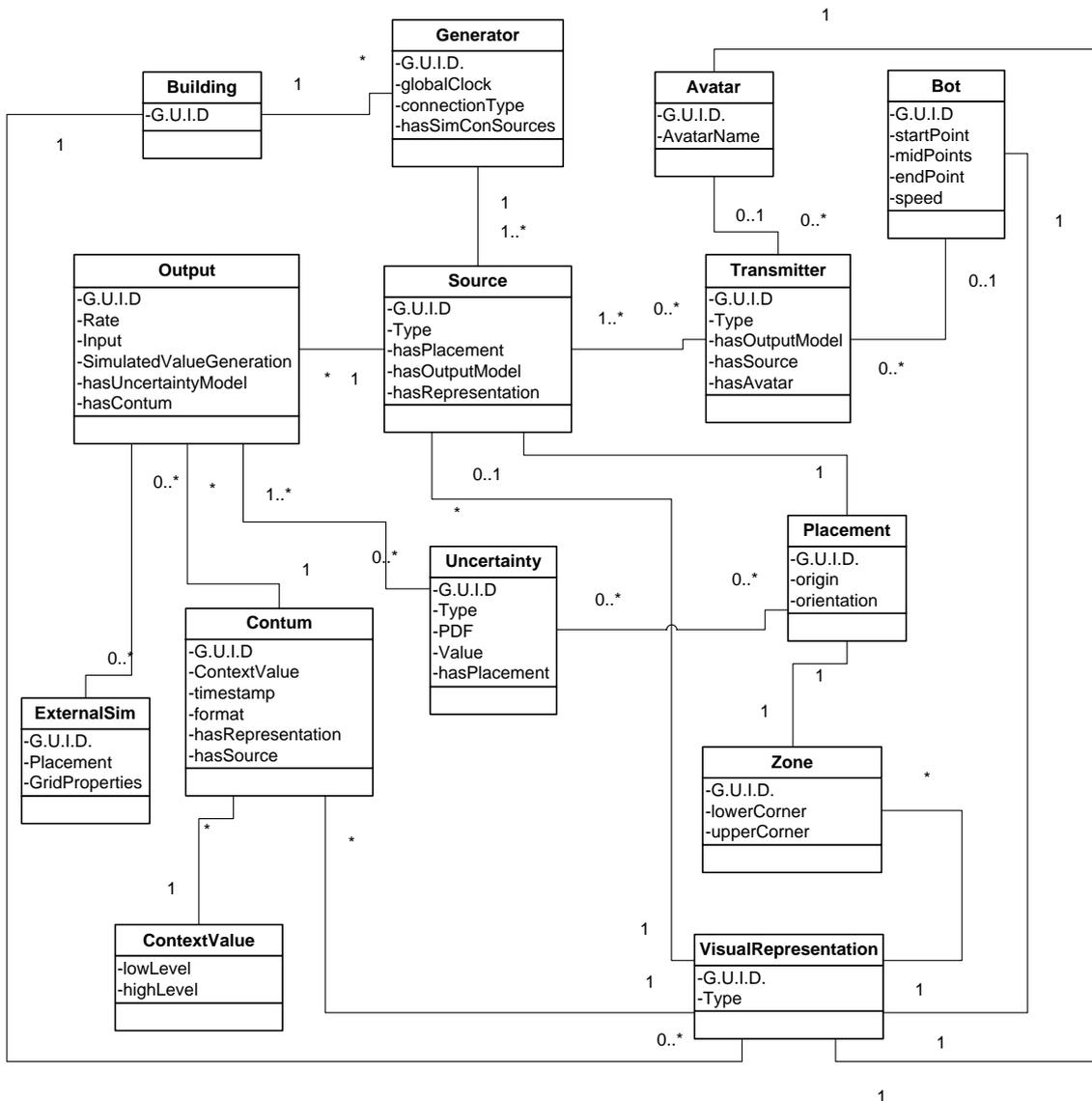
Figure 4-4 UML Class Diagram: SimCon Model
