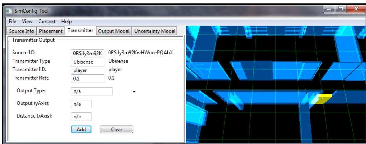
Figure 5-10 Assigning a Ubisense Transmitter to an Avatar named "player" with a transmission rate of 0.1 seconds.
