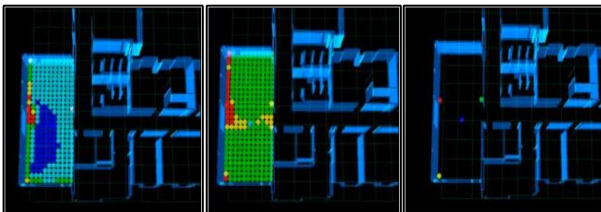
Figure 5-16 External Models for Temperature Simulation, and temperature at point for a room in the NIMBUS centre in Cork. Left centre a heat source has been defined, and an exit right centre an open door.
