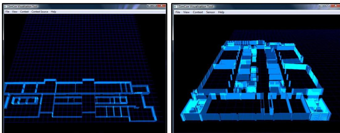
Figure 5-3 Visualisation of Building Model (2D and 2.5D): Supports placement of SimCon sources and also visualisation of contums
