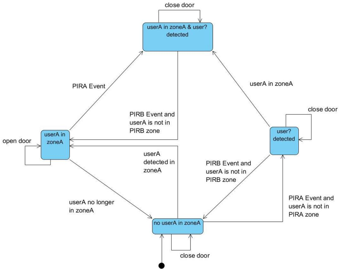
Figure 6-21 Automatic Door Finite State Machine
