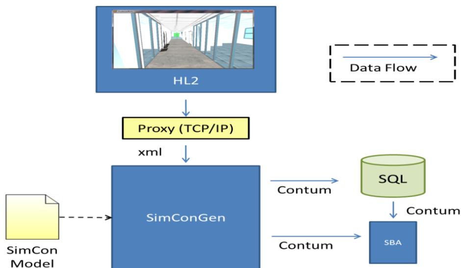
Figure 5-12 Data Communication between the VR Building, the SimCon Generator and the SBA.
