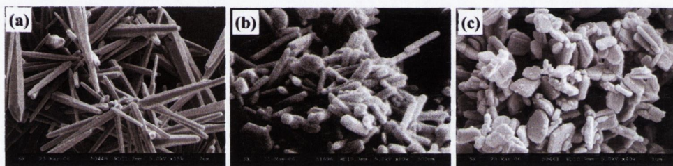
Figure 6.3: SEM pictures of (a) pure ZnO microrods prepared with CTAB, (b) pure ZnO nanorods prepared with ethylenediamine, and (c) Co -doped ZnO platelets prepared with CTAB.
