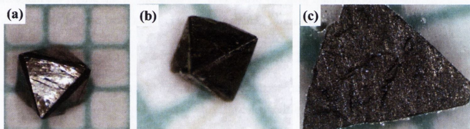
Figure 4.6: Single crystal of (a) pure CdCr_2Se_4 , (b) Ag -doped CdCr_2Se_4 , and (c) cut along the [111] direction of a CdCr_2Se_4 crystal showing the traces of inclusions. The grid has a 1 mm scale.
