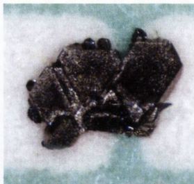
Figure 4.7: Pure CuCr_2Se_4 single crystal grown by CVT using Se as transport agent.
