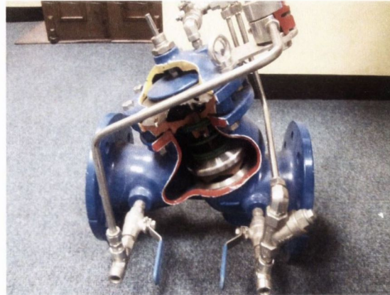
Fig. 2.4: Section View of a PRV
