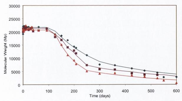
Figure 9.2 Influence of particle size on the molecular weight profiles of PLA (R203) particles incubated at pH 7.4 and 37°C, where ◆ <1 micron, ■ <20 micron and ▲<50micron particles (data points represent mean of two determinations). Data fitted to Equation 8.2.
