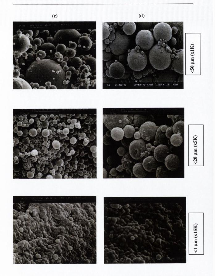
Figure 7.7 Electron micrographs of PLGA particles after incubation in PBS pH7.4 at 37°C, for (c) 11 days (d) 15 days.
