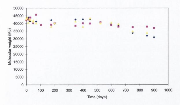
Figure 8.26 Molecular weight profile for PLGA particles incubated in phosphate buffer saline pH 7.4 at  $5^{\circ}$ C, where 4 < 1 micron 4 < 20 micron and 4 < 50 microns (data points represent the mean of two samples).
