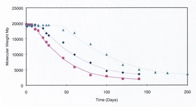
Figure 10.5 The influence of %w/w fluphenazine loading on the degradation of the PLA (R203) microspheres, for ▲ 4.50 %, ◆ 9.86 % and ■ 16.81% fluphenazine loaded microspheres (data points represent mean of two determinations). Data points fitted to Equation 8.2.
