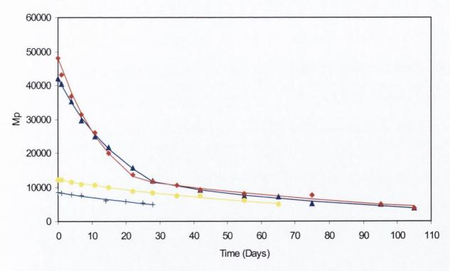
Figure 8.9 Influence of polymer end group on the degradation of PLGA microspheres incubated at 37°C and pH 7.4, for ▲ RG504, ◆ RG504H, ○ RG502 and × RG502H particles (data points represent the mean of two determinations). Data points fitted to Equation 7.3.
