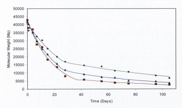
Figure 7.3 Influence of particle size on the molecular weight profiles of PLGA (RG504) particles incubated at pH 7.4 and 37°C, for ◆ < 1 micron, ▲ <20 microns and ■ <50 microns particles (data points represent mean of two samples). Data points fitted to equation 7.3.
