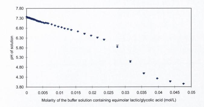
Figure 7.13 The effect of addition of a d,l-lactic/Glycolic acid solution on the pH of a phosphate buffer saline (mean of three determinations  $\pm$  standard deviation).
