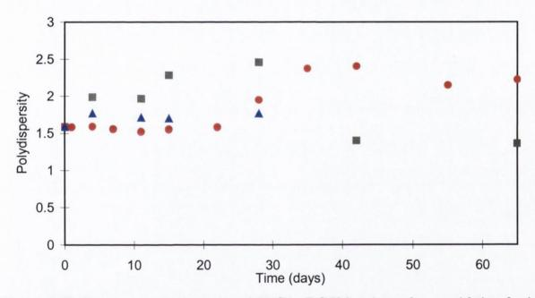
Figure 8.17 Change in polydispersity of PLGA (RG504) microspheres with incubation time, for ● pH 7.4 ▲ pH 10.0 ■ pH 1.0 media (data points represent mean of two samples).
