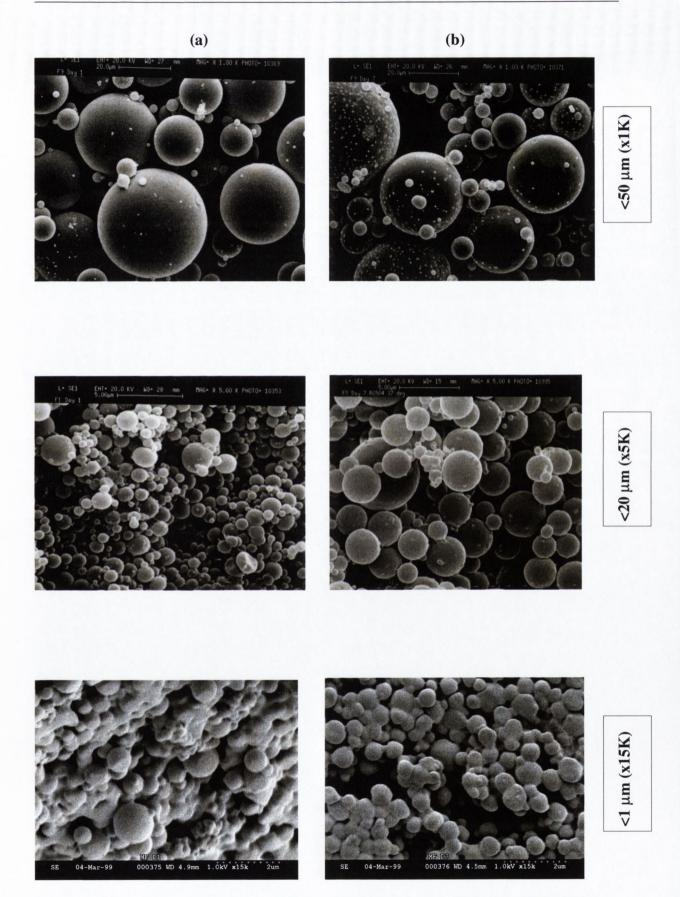
Figure 7.7 Electron micrographs of PLGA particles after incubation in PBS pH7.4 buffer saline at 37°C, for (a) 1 day (b) 7 days.
