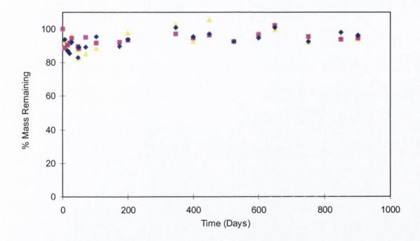
Figure 8.27 Mass loss profile for PLGA (RG504) particles incubated in phosphate buffer saline pH 7.4 at  $5^{\circ}$ C, where 4 < 1 micron 4 < 20 micron and 4 < 50 microns (data points represent the mean of two samples).
