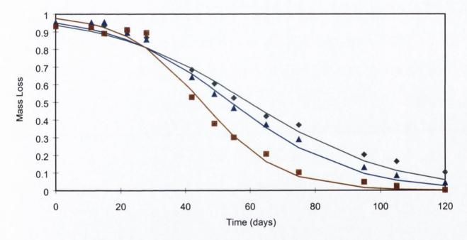
Figure 7.6 Mass loss from PLGA (RG504) particles incubated in PBS at 37°C, for ◆ < 1 micron, ▲ <20 micron and ■ <50 micron particles (data points represent mean of two samples). Data points fitted to Equation 3.23.
