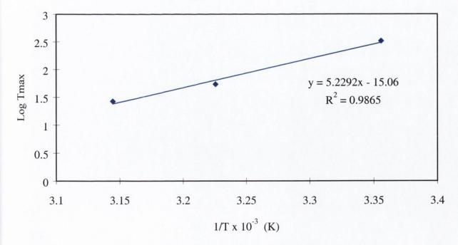
Figure 8.22 Arrhenius plots for the degradation of RG504 microspheres using *Tmax* determined using the Prout-Tompkins equation (Equation 3.23).
