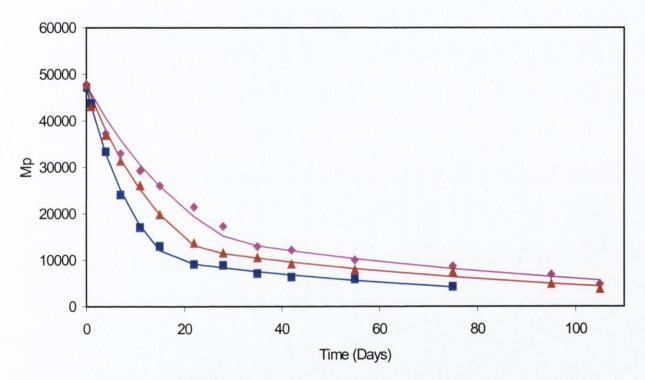
Figure 8.11 Plots of polymer Mp with incubation time for different particle size RG504H microspheres, for ◆ <1 micron ▲ <20micron ■ <50micron particles (data points represent mean of two determinations). Data points fitted to Equation 7.3.
