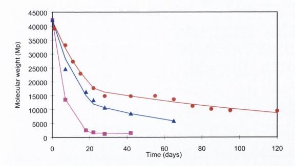
Figure 7.14 The effect of d,l-lactic/glycolic acid concentration on the degradation of 100mg of PLGA microspheres, for ● 0 M ▲ 0.012M ■ 12 M d,l-lactic/glycolic acid (data points represent mean of two determinations). Data points fitted to Equation 7.3.
