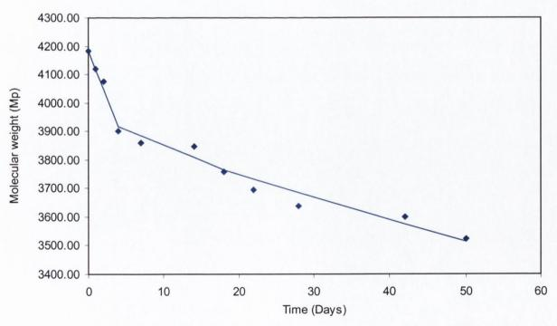
Figure 9.9 The degradation profile of PLA R104 microspheres (<20microns) in phosphate buffer saline pH 7.4 at 37°C fitted to Equation 7.3 (data points represent mean of two determinations).
