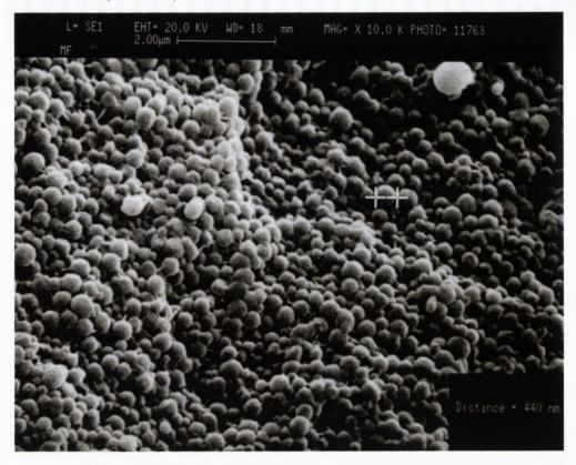
Figure 6.3.2 Electron micrographs of PLA(R203) particles prepared using different modifications of the solvent evaporation procedure (a) Spray dried (b) Stirred at 1,200 rpm (c) Probe sonicated (d) Homogenised at 24,000 rpm and (e) Microfluidised.
