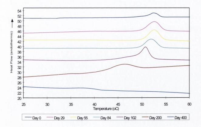
Figure 8.23 DSC thermograms of the degradation of PLGA (RG504) microspheres (<20 microns) incubated at 25°C in phosphate buffer saline pH 7.4.
