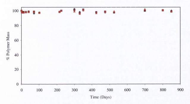
Figure 9.8 Influence of particle size on the weight loss of PLA particles incubated at pH 7.4 and 5°C, for ◆ <1 micron, ■ <20 micron and ▲<50micron particles (data points represent the mean of two determinations).
