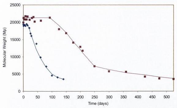
Figure 10.6 The influence of fluphenazine on the degradation of PLA (R203) microspheres, for ◆ 9.9% w/w fluphenazine HCl loaded PLA microspheres and ■ drug free PLA microspheres (data points represent mean of two determinations). Data points fitted to Equation 8.2.
