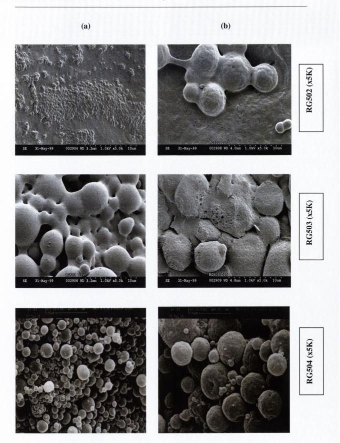
Figure 8.5 Electron micrographs of PLGA microspheres of different molecular weights after (a) 11 days and (b) 15 days incubation in PBS pH 7.4 at  $37^{\circ}$ C.
