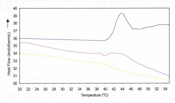
Figure 8.8 DSC thermograms of PLGA microspheres after incubation for 28 days in PBS pH 7.4 at 37°C, for \_\_\_\_ RG504 \_\_\_\_ RG503 and \_\_\_\_ RG502 particles.
