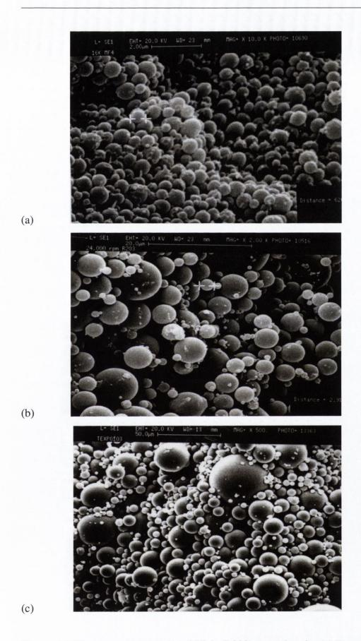
**Figure 9.1 Electron micrographs of PLA (R203) particles,** for (a) Process A (b) Process B (c) Process C.
