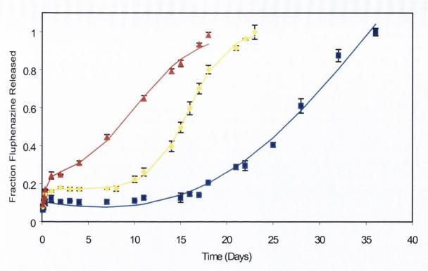
Figure 10.4 Influence of fluphenazine loading (w/w) on the release from PLGA (RG504) microspheres at 37°C in phosphate buffer saline pH 7.4, for ■ 4.50%, ◆ 9.86% and ▲16.81% fluphenazine loaded microspheres (data points represent mean of three determinations ± standard deviation). Data points fitted to Equation 10.1.
