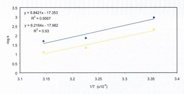
Figure 8.19. Arrhenius plots for the degradation of PLGA (RG504) microspheres, where \_\_\_ k<sub>1</sub> and \_\_\_ k<sub>2</sub> degradation rate constants for PLGA(RG504).
