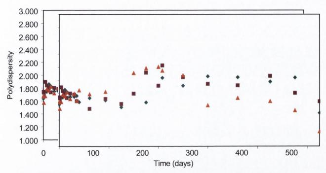
Figure 9.3 Evolution of polydispersity with incubation time for PLA R203 particles, for ◆ <1 micron, ■ <20 microns and ▲ <50microns (data points represent mean of two determinations).
