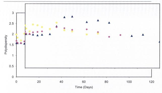
Figure 8.3 Evolution of the molecular weight distribution for the degradation of PLGA of different starting molecular weights, for ▲ RG504, ◆ RG503 and ○ RG502 particles (data represent the mean of two determinations).
