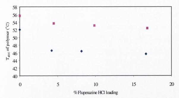
Figure 10.2 The influence of fluphenazine HCl on the  $T_{g(p)}$  of PLA and PLGA polymer microspheres, for  $\blacksquare$  PLA (R203)  $\spadesuit$  PLGA (RG504) microspheres.
