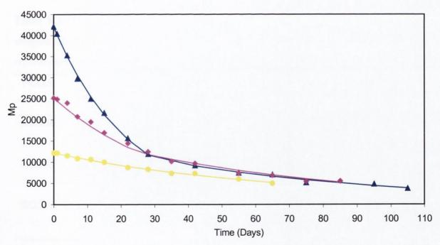
Figure 8.2 Influence of polymer molecular weight on the degradation of PLGA microspheres, for ▲ RG504, ◆ RG503 and ○ RG502 particles (data points represent mean of two determinations). Data points fitted to Equation 7.3.
