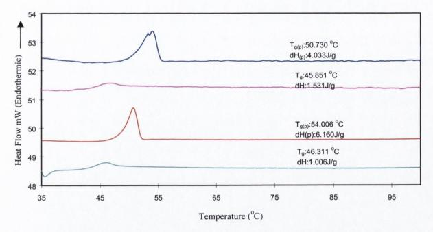
Figure 6.3 The DSC thermograms of PLA (R203) and PLGA (RG504) first heat (Run 1) followed by sample cooling then a second heat (Run 2), for \_\_\_ PLGA (Run 1), \_\_\_ PLGA (Run 1) and \_\_\_ PLA (Run 2).
