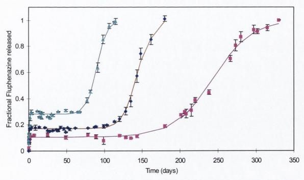
Figure 10.3 Influence of fluphenazine loading (w/w) on the release from PLA (R203) microspheres at 37°C in phosphate buffer saline pH 7.4, for  $\blacksquare$  4.5%,  $\blacklozenge$  9.9 % and  $\blacktriangle$  16.8% fluphenazine loaded microspheres (data points represent mean of three determinations  $\pm$  standard deviation). Data points fitted to Equation 10.1.
