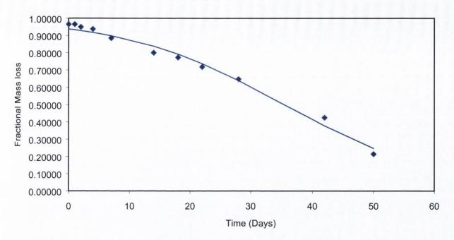
Figure 9.11 The degradation profile of PLA R104 microspheres (<20microns) in phosphate buffer saline pH 7.4 at 37°C (data points represent the mean of two determinations). Data fitted to Equation 3.23.
