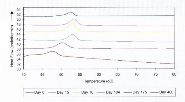
Figure 8.28 DSC thermograms of PLGA (RG504) microspheres incubated at 5°C in phosphate buffer saline pH 7.4
