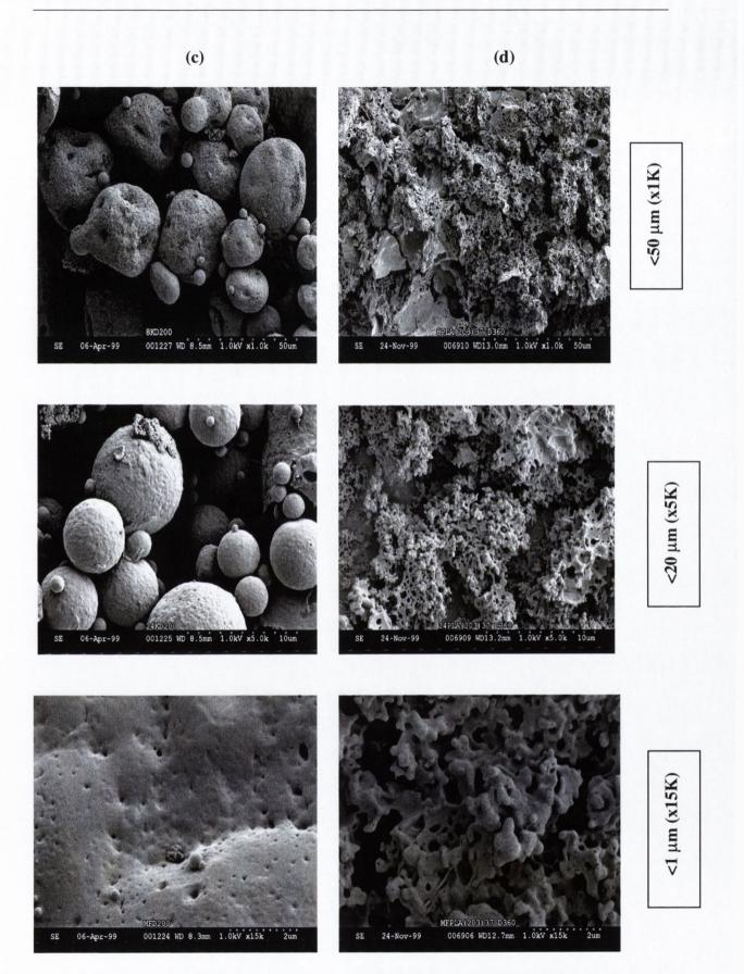
Figure 9.5 Electron micrographs of PLA (R203) particles after incubation in phosphate buffer saline at 37°C, for (c) 200 days and (d) 350 days.
