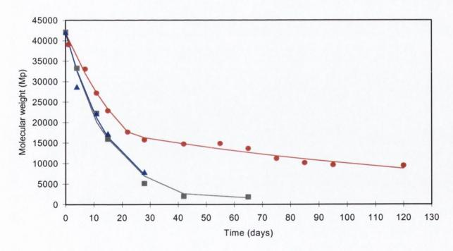
Figure 8.14 Influence of incubation medium pH on the degradation rate of PLGA microspheres (<20 microns) at 37°C, for ● pH 7.4, ▲ pH 10.0 and ■ pH 1.0 media (data points represent mean of two samples).
