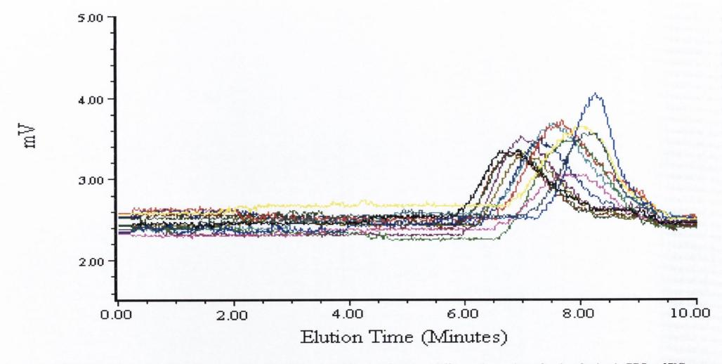
Figure 7.4 GPC Chromatograms of PLGA microspheres (<20 microns) after incubation at different time points after incubation in PBS at 37°C
