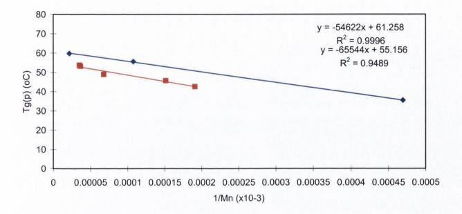
Figure 6.4 Flory-Fox plots for PLA and PLGA polymers, for ■ PLGA Series and ▲ PLA series data points (data fitted using linear regression).
