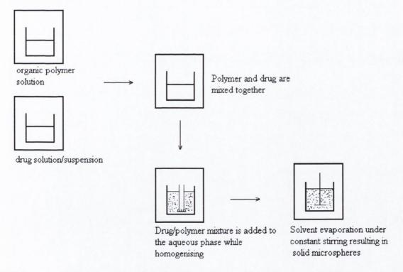
Figure 2.1 Schematic diagram of a basic solvent evaporation procedure
