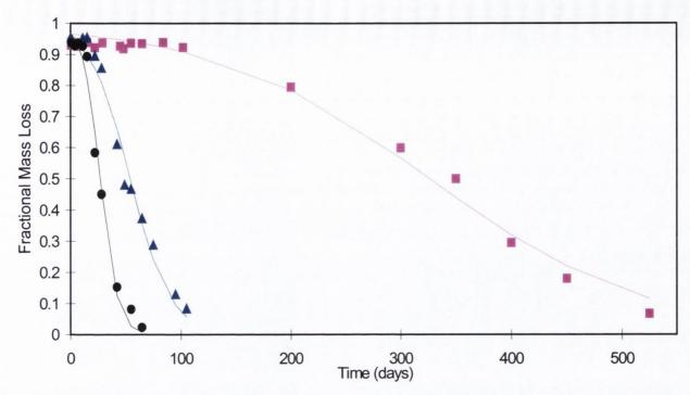
Figure 8.20 Effect of incubation temperature on the mass loss from PLGA(RG504) microspheres, for ● 45°C, ▲ 37°C, and ■ 25°C temperatures (data points represent mean of two samples). Data points fitted to Equation 3.23.
