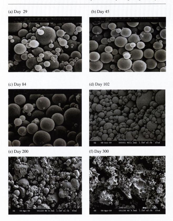
Figure 8.25 The evolution of microsphere morphology with the degradation for PLGA (RG504) microspheres incubated at  $25^{\circ}$ C.
