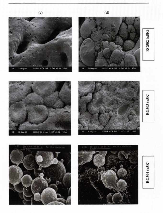
Figure 8.5 Electron micrographs of PLGA microspheres of different molecular weights after (c) 22 days and (d) 28 days incubation in PBS pH 7.4 at 37°C.
