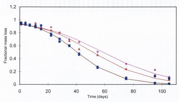
Figure 8.13 Weight loss of PLGA (RG504H) particles at 37°C and pH 7.4, for ◆ <1 micron, ▲ <20micron and ■ <50micron particles (data points represent mean of two determinations). Data points fitted to Equation 3.23.
