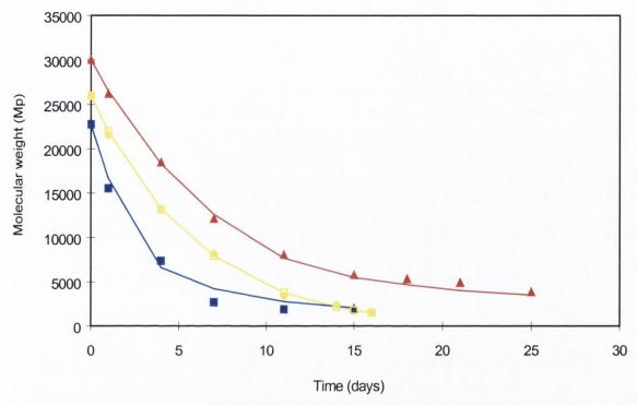
Figure 10.7 The influence of Fluphenazine loading (w/w) on the degradation of the PLGA (RG504) microspheres at 37°C in PBS pH 7.4, for ▲ 4.5 %, ◆ 9.9 % and ■ 16.8% Fluphanazine loaded microspheres(data points represent mean of two determinations). Data points fitted to Equation 7.3.
