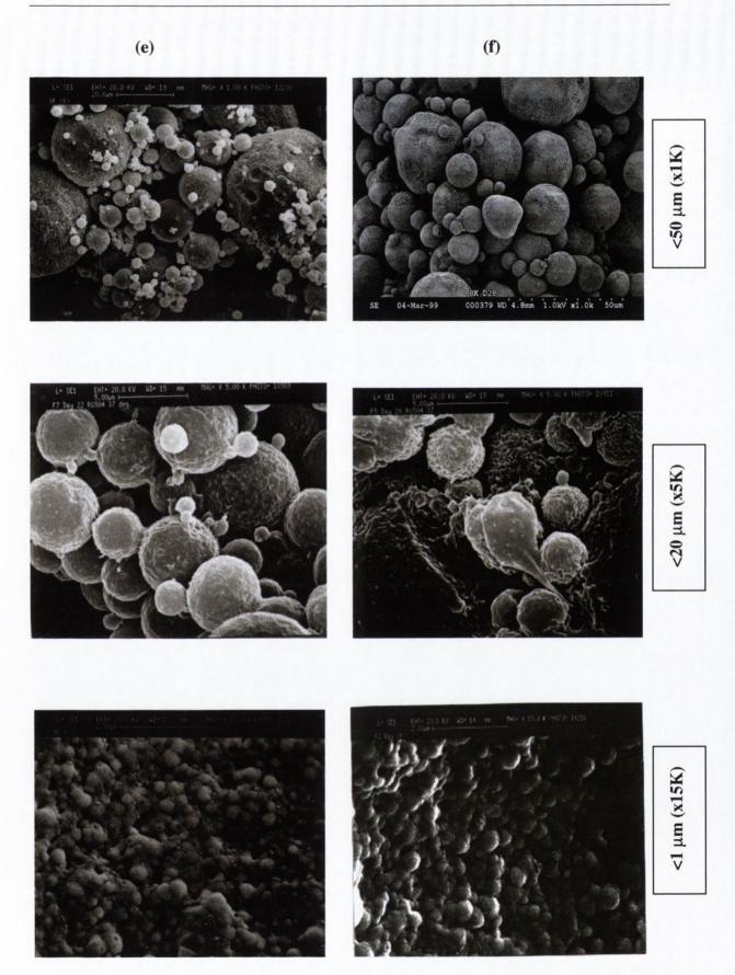
Figure 7.7 Electron micrographs of PLGA particles after incubation in PBS pH7.4 at 37°C, for (e) 22 days (f) 28 days.
