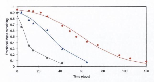
Figure 8.15 Influence of incubation medium pH on the mass loss from PLGA(RG504) microspheres (<20 micros) at 37°C, for ● pH 7.4, ▲ pH 10.0, and ■ pH 1.0 media (data points represent mean of two samples). Data points are fitted to Equation 3.23.
