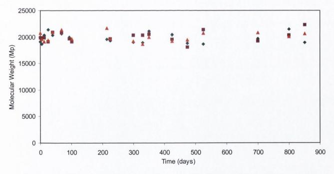
Figure 9.7 Influence of particle size on the molecular weight profiles of PLA particles incubated at pH 7.4 and 5°C, for ◆ <1 micron, ■ <20 micron and ▲ <50 micron particles (data points represent the mean of two determinations).
