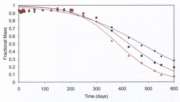
Figure 9.4 Weight loss of PLA particles at 37°C and pH 7.4, for ◆ <1 micron ■ <20 micron ▲ <50micron particles (data points represent mean of two determinations). Data fitted to Equation 3.23.
