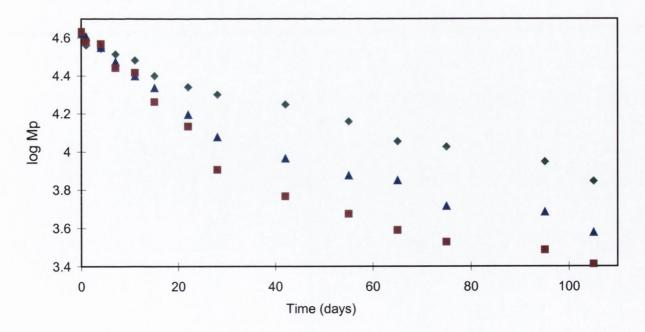
Figure 7.2 Plots of log molecular weight (Mp) with incubation time for PLGA (RG504) particles incubated in PBS pH 7.4 at 37°C, for ◆ < 1 micron, ▲ <20 micron and ■ <50 micron particles (data points represent mean of two samples).
