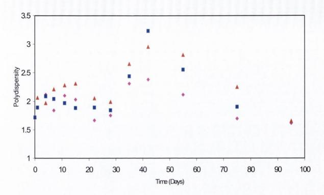
Figure 8.12 Evolution of the polydispersity with degradation time for PLGA RG504H particles incubated at 37°C in Phosphate buffer saline, for ◆ <1 micron, ▲ <20micron and ■ <50micron particles (data points represent mean of two determinations).
