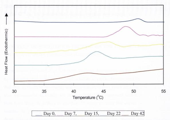
Figure 7.9 DSC thermograms of dried PLGA microparticles (<  $20\mu m$ ) taken after various incubation time-points in PBS at  $37^{\circ}C$ .
