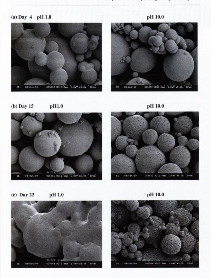
Figure 8.16 Electron micrographs of PLGA RG504 microspheres (<20 microns) incubated in pH 1.0 and 10.0 media for 4, 15 and 22 days at  $37^{\circ}$ C.
