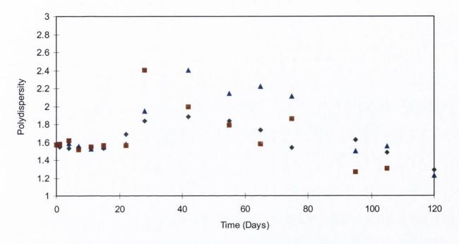
Figure 7.5 Plots of polydispersity as a function incubation time for PLGA (RG504) particles incubated in PBS pH 7.4 at 37°C, for ◆ < 1 micron, ▲ <20 micron and ■ <50 micron particles (data points represent mean of two samples).
