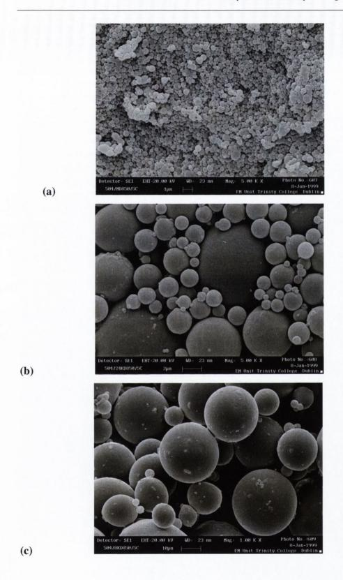
Figure 8.29 Scanning electron micrographs of particles incubated for 850 days at 5°C in phosphate buffer saline, for (a) <1 micron (b) <20 microns (c) <50 microns particles.
