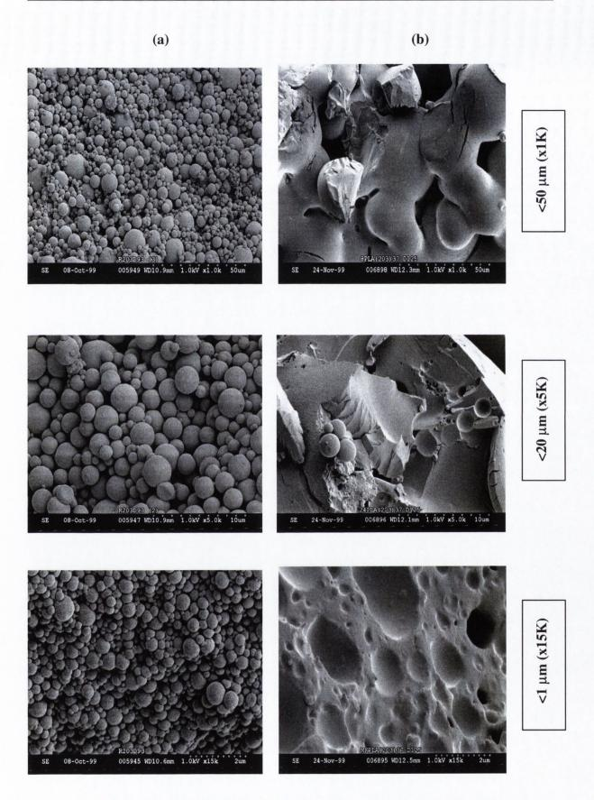
Figure 9.5 Electron micrographs of PLA (R203) particles after incubation in phosphate buffer saline at 37°C, for (a) 93 days and (b) 125 days.
