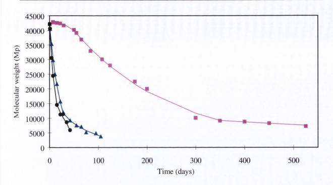
Figure 8.18 Effect of incubation medium temperature on the degradation of PLGA(RG504) microspheres, for ● 45°C, ▲ 37°C and ■ 25°C temperatures (data points represent mean of two samples). Data points fitted to Equation 7.3 or 8.1.
