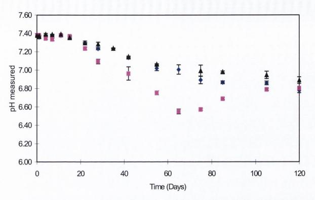
Figure 7.12 The pH profile of PLGA microsphere (Process B) degradation in phosphate buffer saline at 37°C, for ◆ pH of incubation medium containing dispersed microspheres ■ pH measured inside the visking bag ▲ pH of the bulk medium outside visking bag (data points represent mean of three determinations ± standard deviation).
