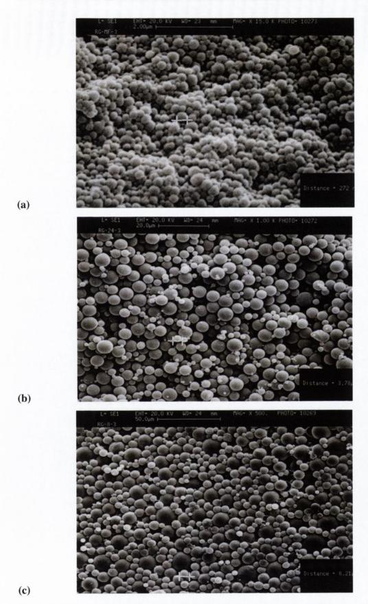
**Figure 7.1 Electron micrographs of PLGA (RG504) particles** (a) Process A (b) Process B and (c) Process C.
