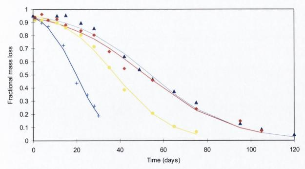
Figure 8.10 Effect of polymer end group on the mass loss from PLGA microspheres at 37°C and pH 7.4, for ▲ RG504, ◆ RG504H, ○ RG502, and × RG502H (data represent the mean of two determinations). Data points fitted to Equation 3.23.
