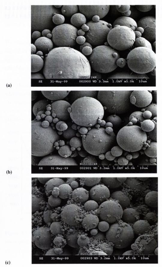
Figure 8.1 Electron micrographs of PLGA particles made from different PLGA molecular weight polymers, for (a) RG504 (b) RG503 and (c) RG502.
