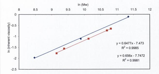
Figure 6.2 Plots of polymer Mw with inherent viscosity, for ■ PLGA series and ▲ PLA series of polymer (data points and fitted using linear regression).
