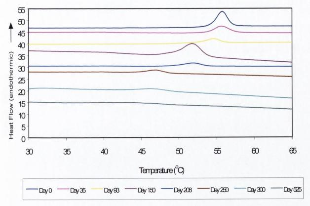
Figure 9.6 DSC thermograms for the degradation of PLA particles (<20 microns) as a function of incubation time in PBS at 37°C.
