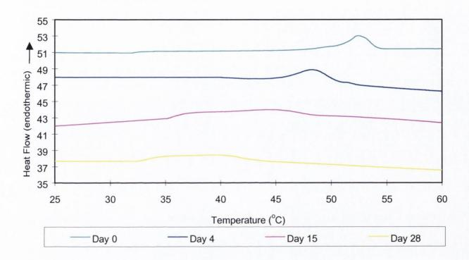
Figure 8.24 DSC thermograms of the degradation of PLGA (RG504) microspheres at 45°C in phosphate buffer saline pH 7.4.
