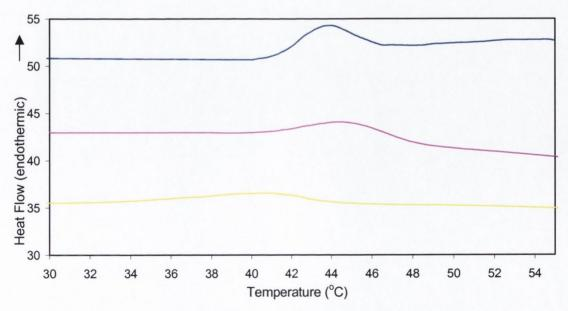
Figure 8.7 DSC thermograms of PLGA microspheres after incubation for 22 days in PBS pH 7.4 at 37°C, for \_\_\_\_ RG504 \_\_\_\_ RG503 and \_\_\_\_ RG502 particles.
