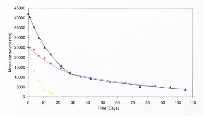
Figure 10.8 The influence of fluphenazine HCl on the degradation of the PLGA microspheres compared to drug free PLGA microspheres, for ▲ drug free RG504, ◆ drug free RG503 and ◆ 8.2 % w/w fluphenazine loaded RG504 (data points represent mean of two determinations). Data points fitted to Equation 7.3.
