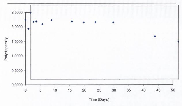
Figure 9.10 Polydispersity profile of PLA R104 microspheres in phosphate buffer saline pH 7.4 at 37°C (data points represent the mean of two determinations).
