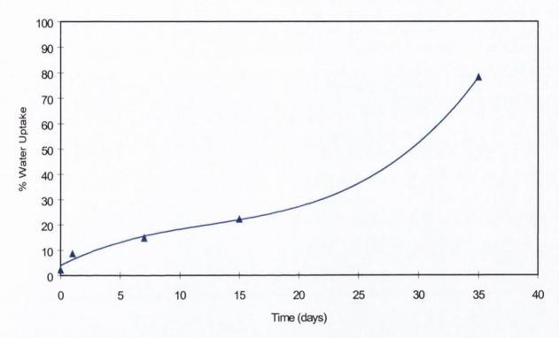
Figure 7.8 Water uptake by microspheres (<20 micron) in PBS pH 7.4 at 37°C as a function of incubation time (samples represent the mean of two determinations).
