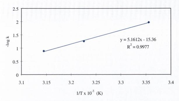
Figure 8.21. Arrhenius plots for the degradation of RG504 microspheres using rate constants determined using the Prout-Tompkins equation (Equation 3.23).
