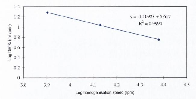
Figure 6.3.1 Log-log relationship between particle size  $D_{50\%}$  and homogenisation speed for the production of PLA(R203) microspheres.
