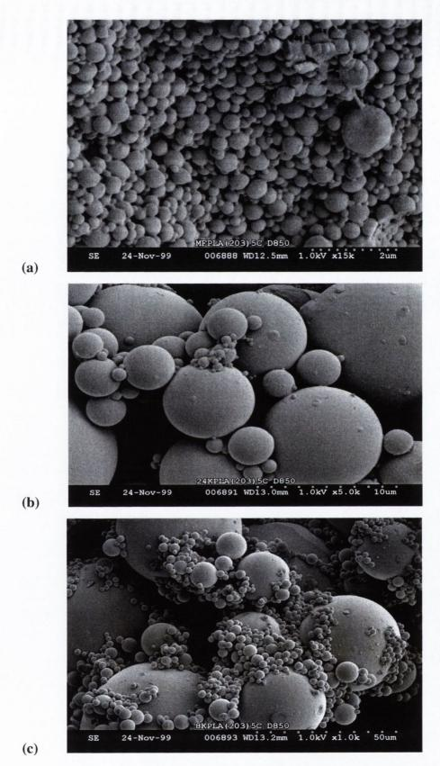
Figure 9.8 Electron micrographs of PLA (R203) particles after incubation for 850 days at pH 7.4 and 5°C, for (a) <1 micron (b) <20 micron and (c) <50 micron particles.
