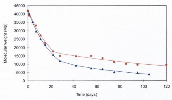
Figure 7.10 A comparison of the degradation profile of PLGA(RG504) microparticles using different dissolution techniques, for ▲ microspheres in visking bags in PBS and ● microspheres dispersed in PBS (data points are based on the mean of two samples). Data points fitted to Equation 7.3.
