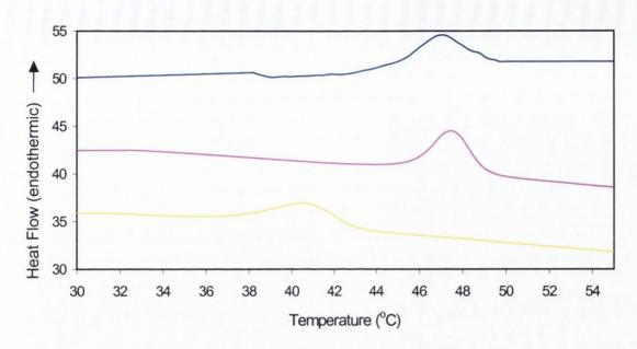
Figure 8.6 DSC thermograms of PLGA microspheres after incubation for 15 days in PBS pH 7.4 at 37°C, for \_\_\_\_ RG504 \_\_\_\_ RG503 and \_\_\_\_ RG502 particles.
