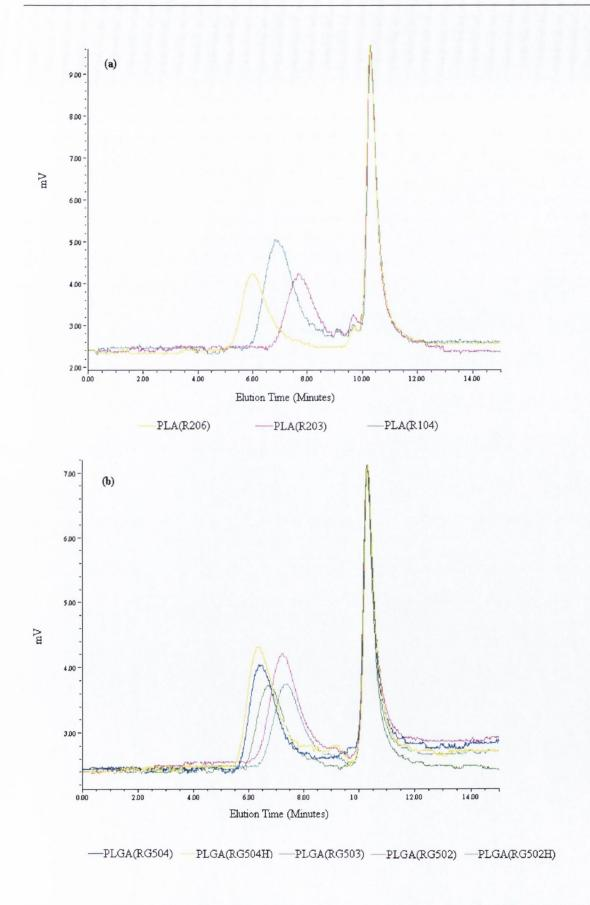
Figure 6.1 Gel permeation chromatograms of a range of poly (alpha-hydroxyl aliphatic esters), for (a) PLA series and (b) PLGA series of polymers.
