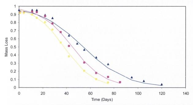
Figure 8.4 Mass loss profiles for the degradation of PLGA microspheres of different polymer molecular weight, for ▲ RG504, ◆ RG503 and ○ RG502 particles (data represent the mean of two determinations). Data points fitted to Equation 3.23.
