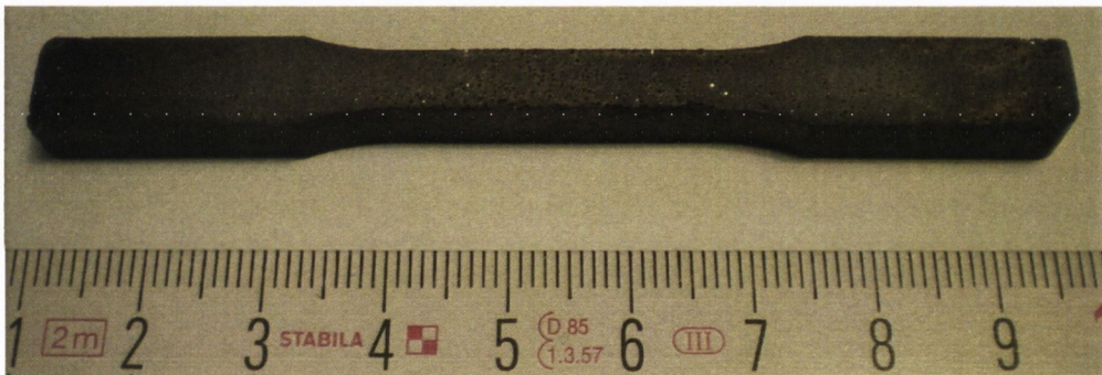
Figure 3.14. Showing a hot pressed tensile specimen; the rough surface shows the diamond crystals protruding on the specimen surface.
