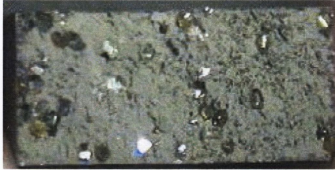
Figure 4.41. TRS specimen showing fracture surface of specimen 30/35 DC40 showing diamonds present on the fracture surface. Run 134/1, mag. x 10.
