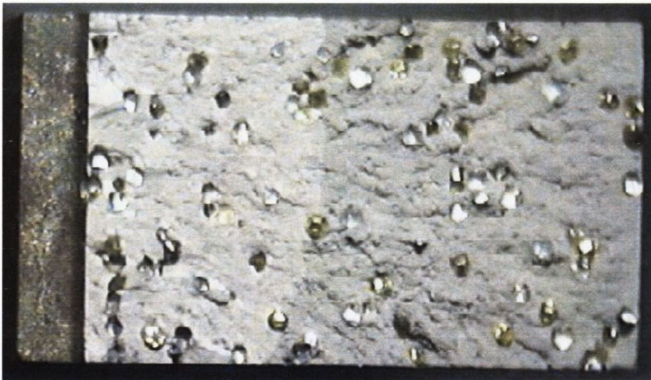
Figure 4.34. FastTrack Fracture Toughness specimen showing fracture surface of specimen 50/60 DC30 showing diamonds present along the fatigue/fast fracture interface. Run 98/1, mag. x 10.
