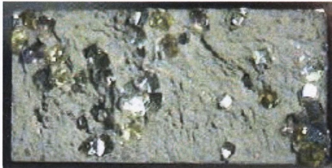
Figure 4.42. TRS specimen showing fracture surface of specimen 25/30 DC40 showing large clustering of diamonds present on the fracture surface. Run 146/2, mag. x 10.
