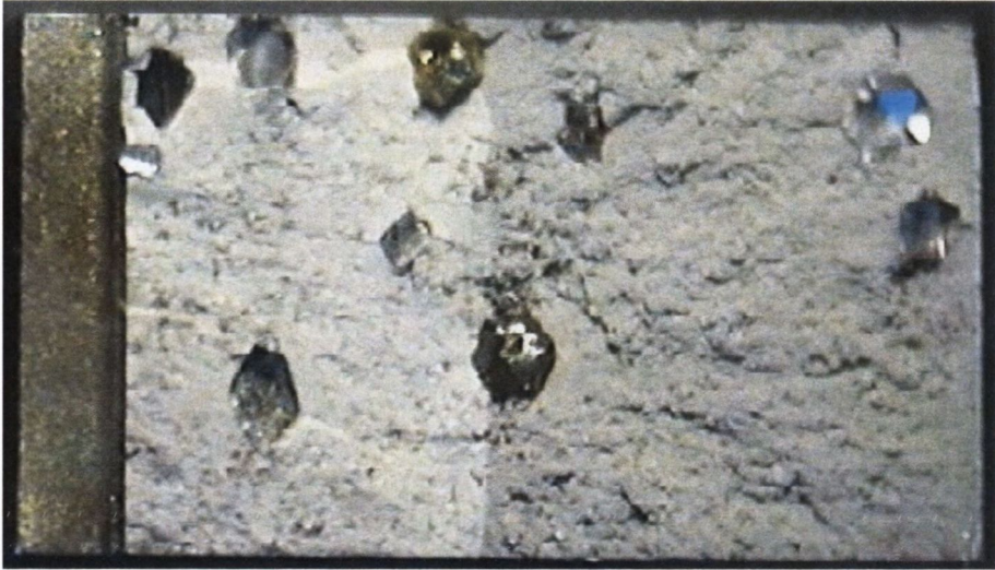
Figure 4.33. FastTrack Fracture Toughness specimen showing fracture surface of specimen 30/35 DC30 showing diamonds present along the fatigue/fast fracture interface. Run 96/3, mag. x 10.
