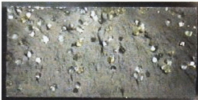
Figure 4.43. TRS specimen showing fracture surface of specimen 45/50 DC30 showing large clustering of diamonds present on the fracture surface. Run 179/2, mag. x 10.
