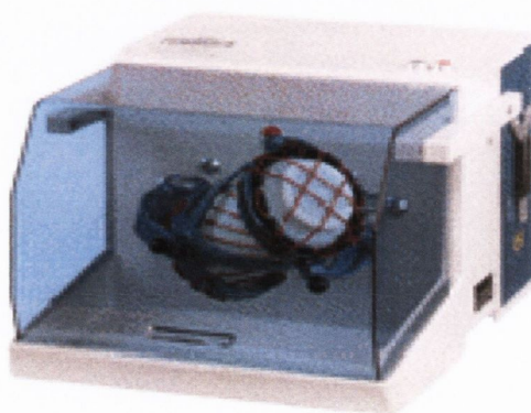
Figure 3.6. Turbula Type Mixer – 'Figure-of-Eight' type mixing motion [227].
