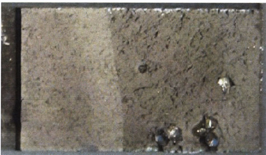
Figure 4.32. FastTrack Fracture Toughness specimen showing fracture surface of specimen 30/35 DC10 showing two diamond clusters present on the fast fracture failure surface. Run 20/6, mag. x 10.
