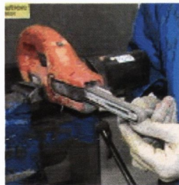
Figure 3.16. Belt grinder used to remove any remaining flashing following hot pressing.
