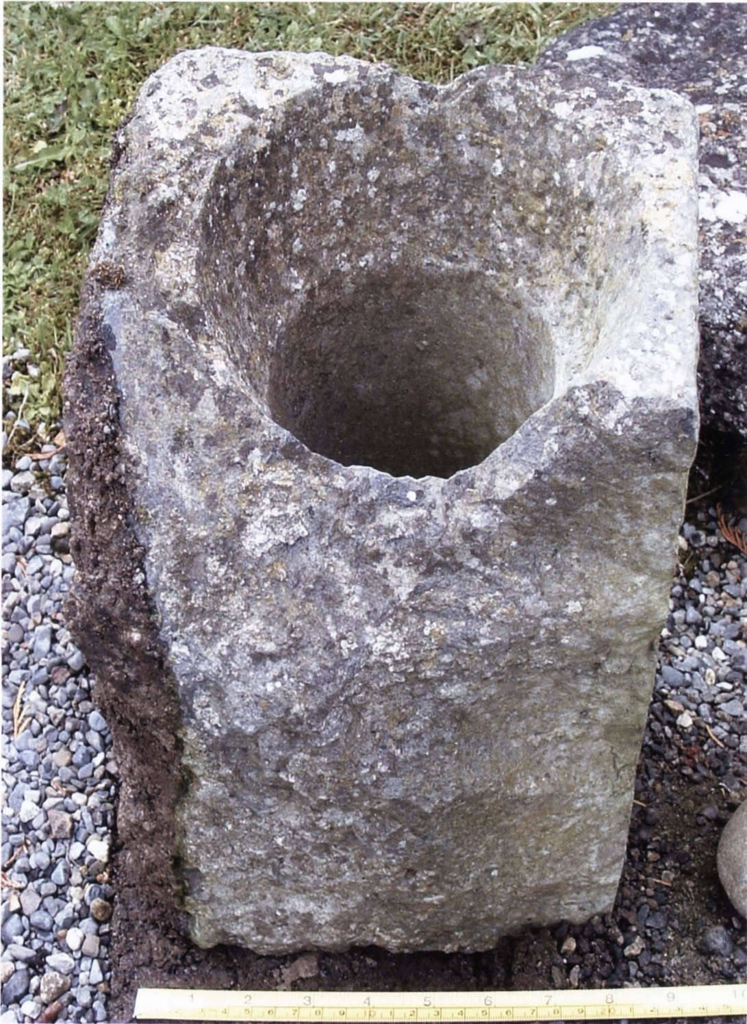
Fig.2.2. Eight inch square section of marble pipe with countersunk head for proper fit to prevent leaking. This section of pipe is from Castlefield House, Co. Kilkenny.
