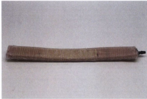
Barbed Vent in Actuator Made with Pin Molding Method - Does not leak up to 40 PSI without SilPoxy. Adding SilPoxy to the hole before inserting the barb produces the best seal after two days - Actuator pops before leaking at that joint.
