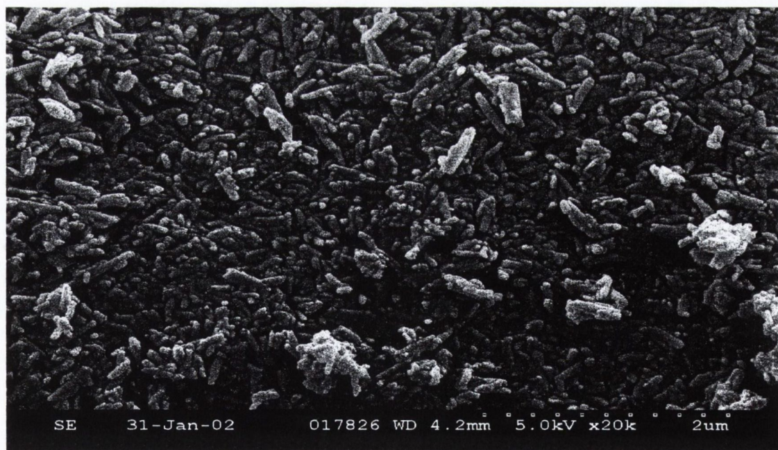
Figure 4.2.2 SEM of halloysite (X20,000).
