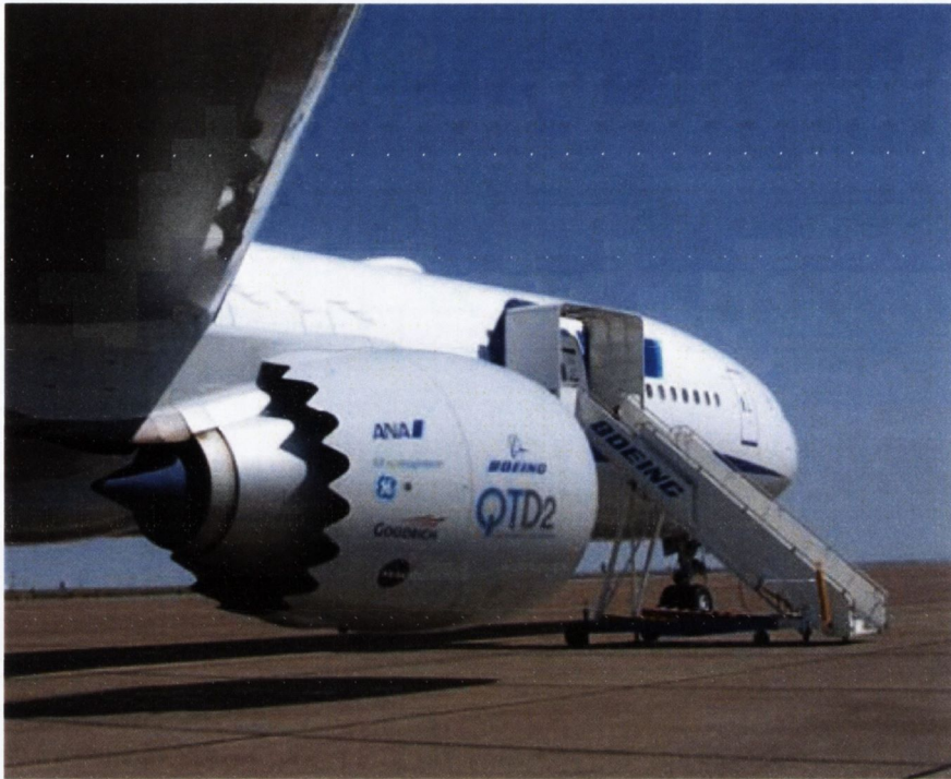
Figure 4.2: Boeing 777-300ER with Chevron Nozzle
