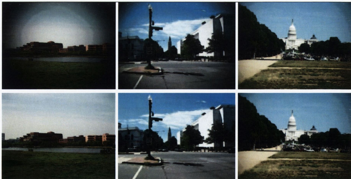
Figure 2.7: (Top row) Degraded images and (Bottom row) and corrections obtained using the technique developed by Zheng et al. [91]. (Images taken from [91])
