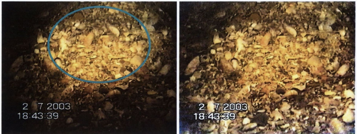
Figure 6.1: Original degraded image on the left with footprint estimate superimposed in blue, and the correction obtained using the proposed method is shown on the right.
