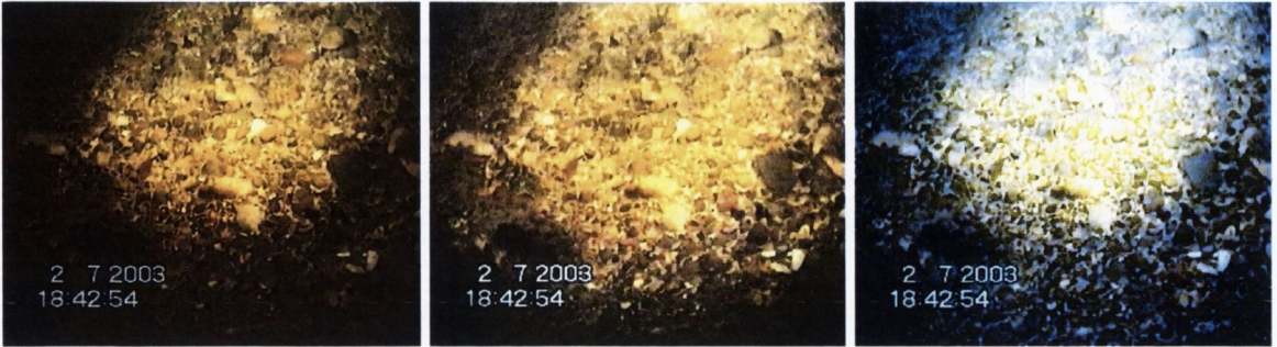
Figure 2.6: (Left) Original degraded underwater image, with the corresponding corrections obtained from the vignetting correction technique of Kim & Pollefeys [45] (Middle), and from using histogram equalization (Right).
